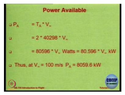
Power available is basically the thrust available into the velocity, thrust available is going to be given to you two engines each of 40298, so therefore it will be 80596 into V infinity in watts which will be 80.596 kilo watts I have just divided by 1000. So total power available is 80 kilo watts so at 100 meter per second the velocity of 100 will give you 8059 kilo watts, required 1127, available 8059, required is only one eighth of available so absolutely no problem, ok.
