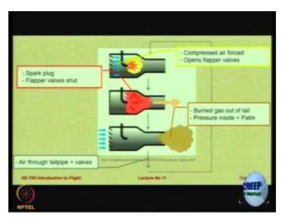
So, here is a working of the pulse jet. The compressed air from the front forces the flapper or butterfly valves open and the timing is very important when you open it at that time only the exhaust the combustion should start. With the combustion the back pressure closes the valves exhaust comes out as it is exhausted out, then air is again sucked in okay. This is what I already told you.
