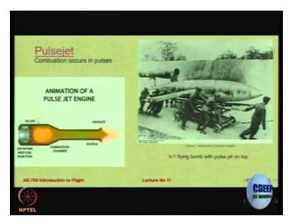
So this is the animation of how a pulse jet works. The key in a pulse jet is the availability of these series of valves in the front, so what do we see here is? If you go in slow motion you will see the air is intake there is an air intake in which air comes in when there comes in because of pressure the valve opens. When it goes inside you ignite, back pressure closes the valve and the reaction throws the product of combustion behind.
