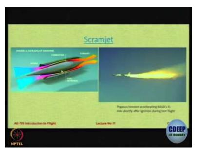
Now, going one step further is the supersonic combustion Ramjet or the Scramjet. And this technology is also under investigation in our country because we are making a vehicle called as the HSTDV. DRDO is working on a project and we are almost near the completion of that particular design. So let us have a look at Scramjet engine and its working.
