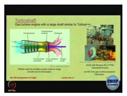
For example this is the world's first helicopter which had a turbofan turbine powered before this helicopters were generally used only piston powered or this was the first one to have a gas turbine in a helicopter and that one was a turbo shaft okay.
