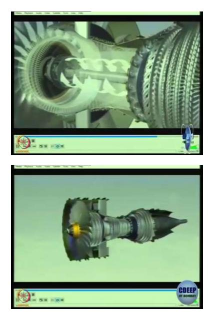
Video: To make an aircraft move forwards we need a pushing force or thrust which we create by making the air accelerate between the front and the back of the engine this is basically giving by the large fan at the front of the engine through which air passes at a high rate these are the various components of the CFM56-7B.
