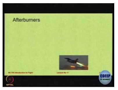
Now if you have a jet engine and if you really want to push the limits and if you want to go for higher thrust then in the exhaust of the jet engine we still have some unburnt air, unburnt oxygen so if you spray fuel in that and ignite it you can get extremely high thrust.
