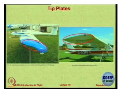
The other way of induce drag management would be, to pro-actively work on the strength of the vortex. The 1 way is to put tip plate. The one on your left, the one with the blue end is called as hoerner wing tip it was given by Sighard Hoerner. And, the one on the right is some kind of a device to create method to reduce wing tip.
