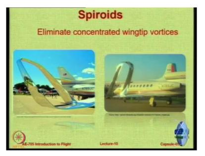
This is another interesting way. Instead of having a tip, just create some kind of a Spiroid. So, you eliminate now there are 2 wing tip, which are joint together. This has been used in many aircraft. As u can see there are practical aircraft with passenger. Which have a very unique kind of wing tip called as a Spiroid tip.
