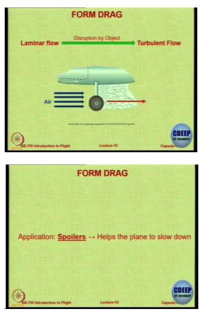
Then form drag can also be because of the disruption. So, by presence of an object the flow becomes turbulent, it could be a protruding rivet or it could be something else. So, you can also have form drag because of the presence of some surface. We have already seen this in first lecture.
