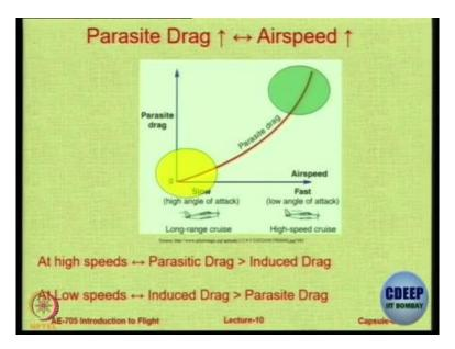
And, this drag increase as the air speed increase. In general if you fly slowly, at a high angle of attack or if, you will higher form drag. But, when you fly fast, at low angle of attack, at that the time rubbing of air on that surface could give you more. So, it depends on which of this term is more in magnitude ok. Generally, at high speed parasite drag is far for more than induced drag.
