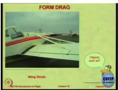
So form drag, very high form drag because of landing gear when it is extended. Very high form drag because of antenna, beacon or, anything projecting out. Also, very high form drag because of object, which are obstructing the flow such as wing struts. Now, tell me why do you think in this aircraft that; you see hear they have used this wing struts. What are the wing strut doing, why are they there, anybody? Here yes.
