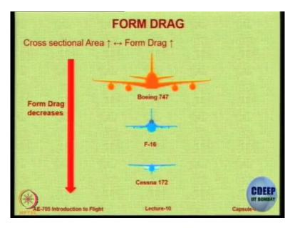
So, as the cross sectional area of the aircraft increase, the form drag will increase. So, from 747 to f16 to Cessna 172 there is a reduction of section area, just by virtue of the size. And, therefore you have a lower form drag ok.
