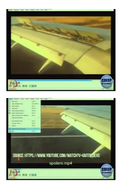
Just after you land you can these thing come up, they create extremely high parasite drag and, that is intentional. Because, at this point we do not want lift, we want to spoil or kill the lift. So, you create high parasite drag by projecting some surface, almost perpendicular to the air stream ok.
