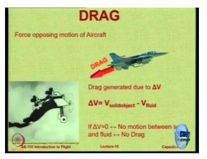
So, drag basically is a force that opposes the motion of the aircraft and it acts only when there is some relative motion between the aircraft and the ambient air. For delta V the relative velocity between the object and the fluid that is needed to create drag, and if there is no relative velocity or if there is no relative motion between the solid and the fluid then there will be no drag.
