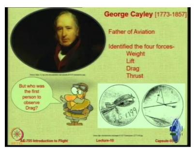
And none another than the father of aeronautics Sir George Caley, in fact, not only drag, he was the first person to talk about the four forces and the proof of this is in a silver coin that was edged in 1799. On one side of the coin was a sketch of Sir George Caley's gliders concept, on the backside was this nice diagram which shows the action of the forces on a flat plate. So, this is a first historical recorded sketch of the four forces acting on any flying body.
