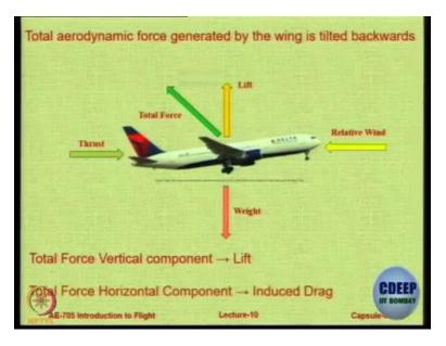
So, you have relative wind on an aircraft you have thrust there is a net reaction but then there is a backward components and that backward component is the induced drag.
