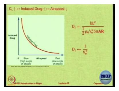
So, if you change the air speed the CL will change, because you need to maintain lift equal to weight still so as the air speed increases the CL will reduce; and if CL reduces,  $\frac{C_L^2}{\pi Ae}$  will come down. So, that is one way of reducing the induced drag, fly faster, ok that is one solution.
