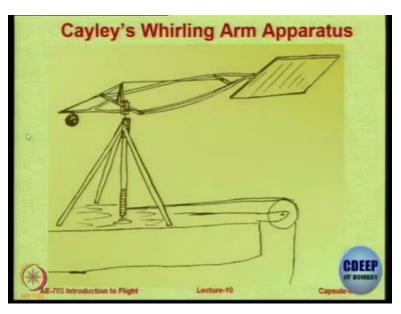
Professor: So, this is a pre curser to the wind tunnels called as the rotary arm or whirling arm apparatus. Such systems were used also to calculate the forces acting on airships and other bodies, ok.
