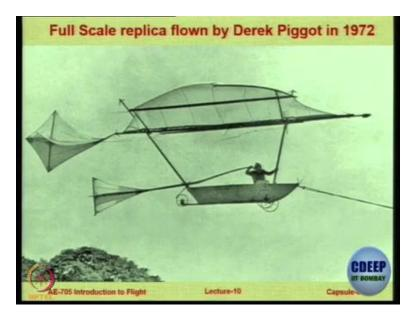
So, here is a picture of the full scale replica of this aircraft, it was flown by Derek Piggot by in 1972 noticed that the radar is hand operated. Now a day, radar is foot operated. But in this particular glider and there is a cable you can see which is attached because it's a glider there is no power plant so you launch it with a cable. So, it was a very successful flight. Ofcourse they did a
