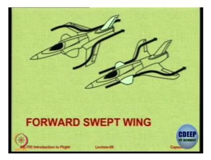
Now, let us look at forward swept wings. Forward swept wings are better than rear swept wings actually speaking because as you can see the Spanwise component is along the, along the root. So therefore, actually the flow is being gathered by the wing on the root and you can make it flow over a controlled surface and make it very-very effective. But there is a problem, there is a problem regarding forward sweep and that problem was encountered by during flight testing.
