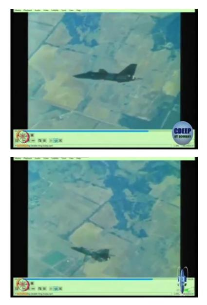
So, during low speed flight lower sweep is better, because you want a high aspect ratio. During high speed flight, it is better to have delta wing or a fully swept wing. So, you go into whatever position is appropriate for your flight profile.
