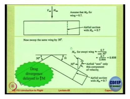
So this is what it is just a repetition. You have an Airfoil which is at M, mach number of 0.7. So, you have no sweep. Therefore, the two sweeps are same. The moment you sweep it, then you have a component and that component (come along) normally is going to reduce. Ok. So, effectively the mach number, the free stream mach number which was 0.7 was critical mach number earlier. It will become 0.808 by a simple approximation. This is only for indication.
