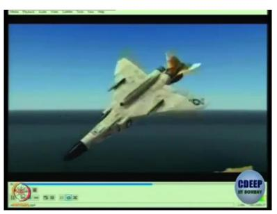
So, inertia coupling happens when two modes of the aircraft start getting coupled and then one of them causes the other to accentuate. And then it becomes completely uncontrollable.
