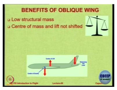
So, there are some benefits, there is a lower structural mass. The center of mass and lift is not shifted. Because on one side it is swept forward, on one side it is swept back. As against either sweep back or sweep forward, the center of gravity is completely shifted ahead. Here it is not shifted. There is a lower wave drag. Let us see, if our video works let us see, how a wave drag is lower?
