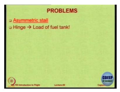
Then the whole wing is going to hinge at one particular point. So, there will be a lot of load on that point. So, that point will be heavily loaded and the place where you are going to, so you imagine you have a wing which carries fuel and then you are moving the whole thing along the hinge. So that is a serious problem. Then we have something called as 'inertia coupling'. Now,
