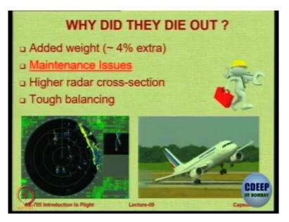
Then you have a higher radar cross section. Because you are providing variable sweep, so under some condition it is going to have low sweep and therefore it will have a much larger cross section. And in some condition it will have a lower one so the if you have a constant high sweep you have a lower cross section. Ok. So, in the next class we are going to look at 'Types of Drag' and what do we do to reduce them. Ok. Thank you.
