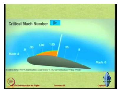
Ok, so this is very clear because of the angle of attack or curvature or camber, there is going to be acceleration of fluid flow both above and below the aerofoil. So, the local Mach number is going to increase from the free stream Mach number. There will be some free stream Mach number at which sonic conditions are first reached anywhere on the aerofoil , remember it could be upper surface, it could be lower surface, it could be front, it could be behind. The lowest free stream
