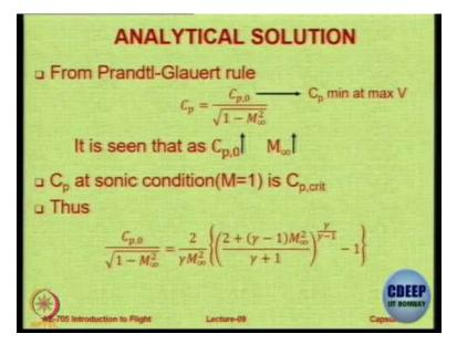
So, what you can do, you can say okay this is a Prandtl Glauert rule and you can notice here that Cp knot is going to increase as M infinity increases or as Cp knot increases the M infinity will increases or vice versa actually, so at sonic conditions so you just equate them at M equal to 1 and by equating them you can actually solve and get the expression, so it is the same thing either you do it graphically or you do it by simultaneous equation.
