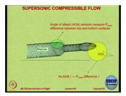
This is the mesh that was created across the pitot-static tube. And the angle of attack sensors mounted, they measure the static differences between the top and bottom surfaces, and with that. So, as the angle of attack increases, then, there is an increase in the static pressure difference. Because of the angle of the pitot-static tube.
