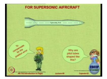
But I want you to see this is a kind of shape that you will see for a pitot-static tube used on all aircraft which go faster than speed of sound. In supersonic flow, so there will be a center symmetry axis and there will be a bulbous nose in the front and there will also be something on the back; So, the question is, why are the pitot tubes shaped like this in case of supersonic aircraft?
