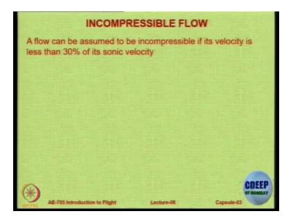
We know from our previous lectures that there is no hard and fast number at which the flow becomes compressible but typically we say that at Mach number 0.3 or lower, you can assume that the flow is incompressible without much error. The errors would be only around 4 to 5 percent at Mach 0.3.
