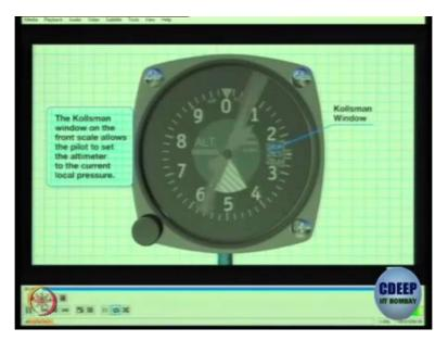
So, you can see that the static port is connected to this instrument from the back and what it simply does is that as the pressure increases, it is going to push this aneroid barometer type bellows and that motion is transmitted through links to the scale.
