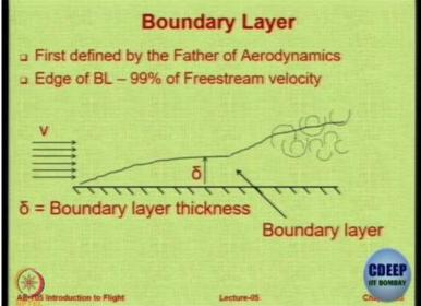
The region in which the viscous flows are predominant is boundary layer and the other region is the normal or the non-boundary layer. So, this is the contribution by the father of aeronautics Ludwig Prandtl and he also gave a definition, where does the boundary layer end? The boundary layer ends when the flow stream velocity inside the boundary layer is almost equal to the free stream velocity.
