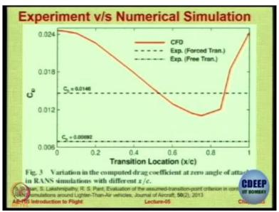
So, the red line that you see is the value of a parameter called drag coefficient for various transition locations, specified intentionally by us. So in the numerical exercise or in the computer program which we have written you can specify transition point. It is not possible in all computer programs; especially if you look at commercial programs you may not be able to do this explicitly. But if you have your own program, you can, ok.
