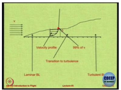
So, here is a full picture of the same thing that we saw earlier, now I have just injected the profile. So, you have a laminar boundary layer in the beginning till there is a transition, and you have these profiles and that red dot basically is the place at which the velocity becomes 0.99 times v infinity, that is why it is called as Delta, the thickness.
