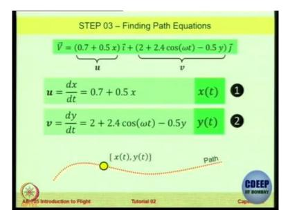
Okay, let us go ahead, so this is the velocity equation. So there is a path which the particle takes and the velocity is going to be a function of x and y which are functions of time. So this is u and that is v okay. So the u is going to be basically
