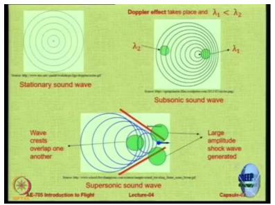
So as we will see now, so this is a stationary sound wave at any point of time there is a sound source and the center and at T equal to 1 unit, you have 1 circle, 2 units, 3 units, 4 units you have these concentric circles. If the source starts moving at a speed that is lower than the speed of sound then you will have still concentric circles but you will find that the gap between them is more on the back and less in the front because the object is also not moving.
