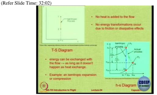
So if it is the process as isentropic then in the T-S diagram it is a straight line, there is no change in s. Ok. Because no heat is added to flow and there is also no energy tranformation because of friction. This is only an assumption, in real life very difficult to get such flows. Okay just a detail. (Refer Slide Time: 32:24)
