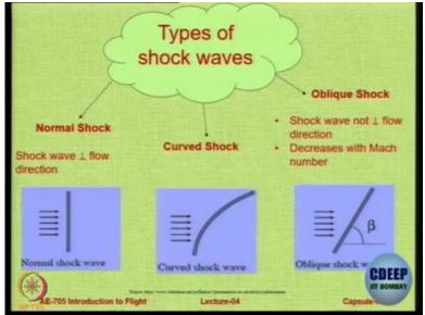
There are 3 or 4 types of shock waves. The first one is a normal shock wave. This is like a front, which moves. This particular kind of shock wave occurs in front of blunt bodies at the in the central region. The next one is an Oblique shockwave. This happens mostly on bodies which are having a very sharp point. So from the point at an angle there will be the shockwaves and this angle beta will depend upon the flow Mach number. You also have curved shock waves. Ok.
