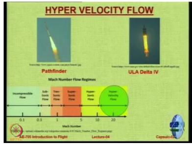
For example, the Pathfinder and the ULA Delta both of which Path finder is basically a missile and ULA Delta 4 is a rocket used to launch satellites. So that is where, now there is nothing like hyper super velocity flow beyond Mach number etcetera. There is no demarcation beyond that. Normally any Mach number beyond 11, 12 we say it is super hyper velocity flow okay. Yes? Student: Sir, Sonic boom also exist in this?
