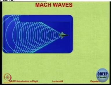
Then there is something called as Mach waves. What are Mach waves? As you can see Mach waves are essentially locus of the intersection of the sonic waves released by an aircraft as it proceeds. Now, since the aircraft is flying higher than speed of sound that is why these the sonic waves the sonic waves are behind the aircraft and they coalesce together and this particular the angle that is created by the intersection of these are is called as a Mach wave.
