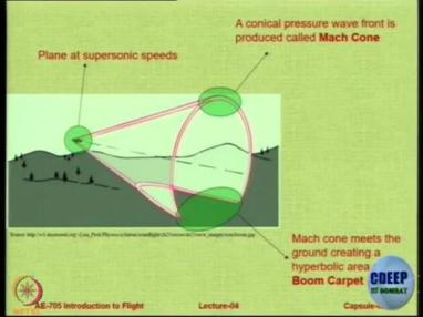
So this creates a parabolic boom carpet. So any and everything that is on that on the ground along that horseshoe type ground interference pattern they are going to be affected by the sonic boom okay.
