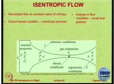
First of all we must look at and understand what is meant by an isentropic flow, it is a flow which is reversible and we assume that there is no entropy loss. It is an assumption. It is very difficult to get in real life any flow where there is no loss in entropy. Entropy the disorder which continuously increases, but for a theoretical calculation purposes or ignoring the loss in the change in the entropy, you can assume the flow to be isentropic.
