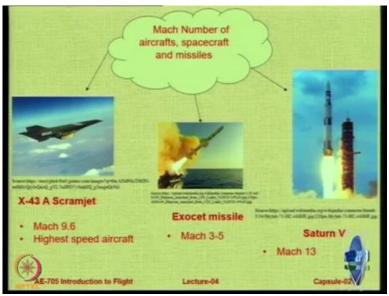
So scramjets operate at around Mach number 10. This is the highest speed aircraft known to human beings. Missiles operate between Mach number 3 to 5 normally and then you have these rockets which go to much higher Mach numbers. The Space Shuttle for example encounters Mach numbers of 20 during its flight. Okay? Ok.
