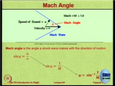
So now the Mach angle or the angle at which the shock wave is inclined at a particular speed is a function of the speed. So you can see very straightforward relationship exists between this Mach angle  $\mu$  and the velocity V and sonic speed *a*. So basically
