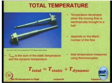
Similarly, we have a concept of total temperature. Again it will be static temperature. But here we have to bring in the effect of Mach number okay. So we use thermocouples to measure the total temperature. So it is the sum of the static temperature and the dynamic temperature again in the same manner as the pressure. Okay.
