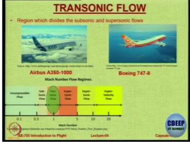
So this is transonic flow regime 0.8 and most aircraft in which we fly long distances for example, Airbus A350 or Boeing 748 they are all transonic flow. They all operate in transonic flow regimes. The typical cruise Mach number will be point 8 for these aircraft.
