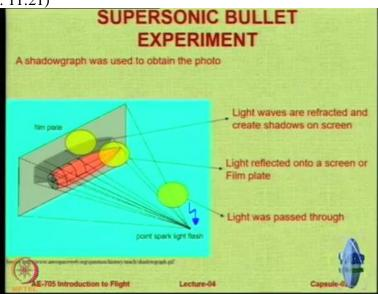
This is a technique that is used to obtain the photo called as a shadow graph, which is different from schlieren. Ok. So light was passed through this particular and there was a reflection on the film plate and then those film plates created shadows and those shadows are what you are seeing. Ok.
