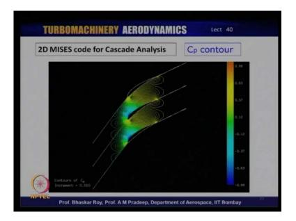
This is an typical output which you finally get of that particular analysis, and here you can see the C p control in terms of the color code that is available; and you can see the pressure of the C p distribution over the entire flow domain, as was described in the last slide. So, this is the out kind of output, you would get, if you do everything properly in a described or prescribed flow domain. This was a two-dimensional cascade flow analysis.
