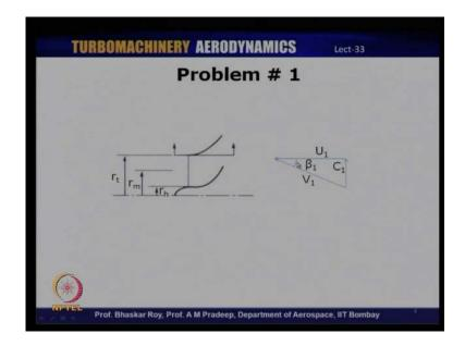
So, let us take a look at the schematic of this particular problem, we have this hub to tip ratio that is been given to us, the radius ratio is 0.4 which means that r h by r t is 0.4. The inlet velocity is given as axial, so C 1 is axial, and then the blade angle beta 1 is one of the parameters we need to calculate, since U 1 is also specified, because we know the tip diameter and the rotational speed, so from there we can calculate the blade angle beta 1.
