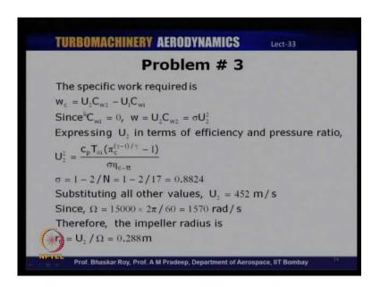
So, the specific work required is U 2 C w2 minus U 1 C w1, C w1 is 0 and therefore, work is U 2 C w2 which is also equal to sigma times U 2 square, because sigma is C w2 by U 2 and so we can express work done in terms of sigma, which is the slip factor and the blade speed at the tip of the impeller U 2, so sigma U 2 square would be the work done - specific work done.
