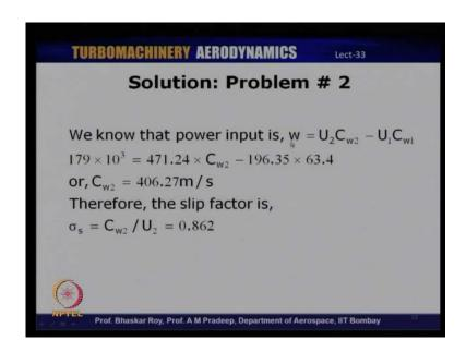
So, let us now calculate C w2 which is the whirl velocity at the tip of the impeller, and since the power work done per unit mass is also equal to U 2 C w2 minus U 1 C w1 and this is equal to work done. We have just calculated earlier 179 kilojoules per kilogram; this is equal to U 2 times C w2 that is 471.24 into C w2 minus U 1 C w1 that is 196.35 into 63.4.
