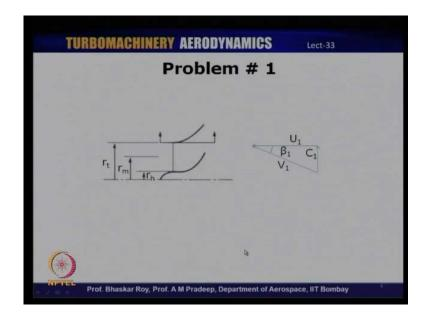
So, if we referred to the velocity triangle we have basically determined C 1, and since U 1 is known you can now calculate beta 1, because it is basically the tan of U 1 and C 1, of course, the first part of the question is also to find the mass flow rate.
