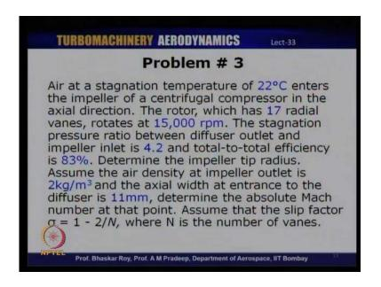
The problem number 3 states that air at a stagnation temperature of 22 degree Celsius enters the impeller of a centrifugal compressor in the axial direction. The rotor, which has 17 radial vanes, rotates at 15000 rpm. The stagnation pressure ratio between the diffuser outlet and the impeller inlet is 4.2 and the total to total efficiency is 0.83 percent or 0.83. Determine the impeller tip radius, assuming that the air density at the impeller
