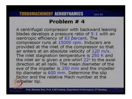
Let us take a look at the problem statement for this question, a centrifugal compressor with a backward leaning blades develops a pressure ratio of 5:1 with an isentropic efficiency of 83 percent. The compressor runs at 15000 rpm. Inducers are provided at the inlet of the compressor. So, that air enters at an absolute velocity of 120 meters per second. The inlet stagnation temperature is 250 Kelvin and the inlet air is given a pre
