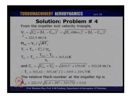
So, from the velocity triangle we see that V 2 is equal to square root of C a square plus U 2 minus C w2 the whole square. So, this C a at the inlet of course, we are assuming that axial velocity does not really change, as it passes through this impeller, this is equal to C a square that is C 1 cos alpha 1 the whole square minus, well, plus U 2 minus C w2 the whole square.
