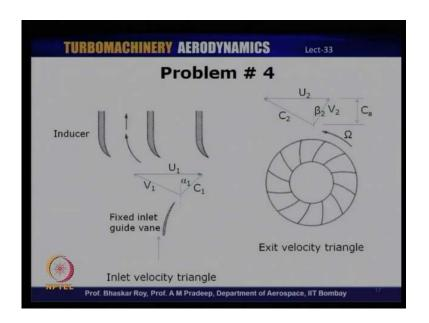
Let us look at the velocity triangles first, both at the inlet as well as the exit, this is the velocity triangle that you should get at the inlet and you have the schematic of the inducer and also fixed inlet guide when which gives a pre whirl to the inlet flow which is entering the inducer.
