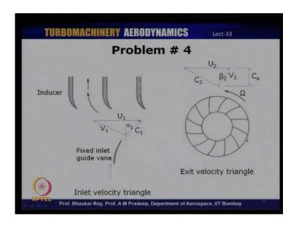
So, the relative Mach number at the tip of the compiler for which we will refer to the velocity triangles once again, let us look at just the velocity exit velocity triangle, for the backward leaning blade we have seen that the velocity triangle would look like this. We have the absolute velocity C 2 and the relative V 2 which is leaving the blades
