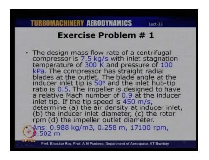
Let us take a look at the first exercise problem, the first exercise problem states that the design mass flow rate of a centrifugal compressor is 7.5 kilograms per second with inlet stagnation temperature of 300 Kelvin and pressure of 100 kilopascal. The compressor has straight radial blades at the outlet, the blade angle at the inducer inlet tip is 50
