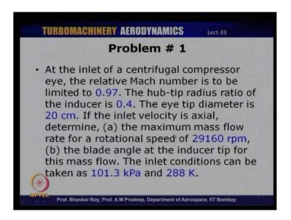
So, the first problem statement is the following, at the inlet of a centrifugal compressor eye, the relative Mach number is to be limited to 0.97. The hub to tip radius ratio of the inducer is 0.4. The eye tip diameter is 20 centimeter and if the inlet velocity is axial, determine, part a - the maximum mass flow rate for a rotational speed of 29160 rpm, part b - the blade angle at the inducer tip for this mass flow. The inlet conditions can be taken as 101.3 kilopascals and 288 kelvin.
