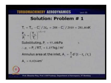
So, let us calculate the mass flow rate, for calculating mass flow rate we need the density, axial velocity is known, we also need the area. Now, the static temperature, you can calculate here because, the stagnation temperature is given, C 1 we have just now calculated, and therefore, static temperature would be 288 minus C 1 square by 2 Cp, C 1
