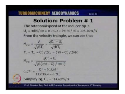
So, if you look at the rotational speed we have been given that the rotational speed is 29160 rpm, diameter is 0.2 - 20 centimeters, so we have phi N by 60 this is 305.36 meters per second. Now, from the velocity triangle we can see that the relative Mach number is basically a relative velocity by square root of gamma R T 1, and at the inlet V 1 is equal to square root of C 1 square plus U 1 square, this divided by square root of gamma R T 1.
