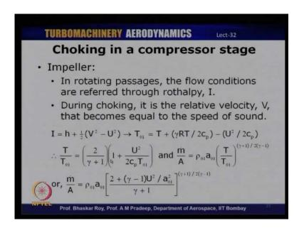
The next component that we will take a look at is the impeller in a rotating passage. As we have seen, the flow conditions are usually referred through the rothalpy, which I had discussed in the last class.
