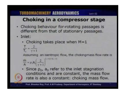
So, choking behavior, because it is different for rotating passages from that of stationary passages, so if you consider the inlet, we know, that of course choking, irrespective of whether it is inlet or impeller, takes places when Mach, the Mach number reaches 1.
