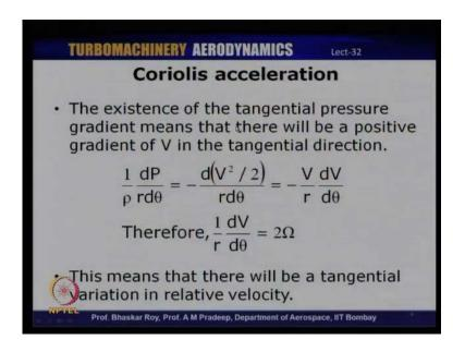
So, if we look at the fact, that there is a tangential pressure gradient, then tangential pressure gradient needs to result in a positive gradient of V in the tangential direction. Because if there is a pressure gradient in a certain direction, that needs to also being the
