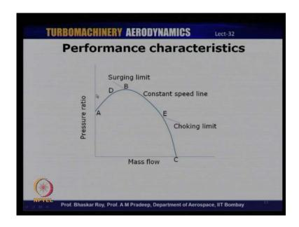
So, if we look at the variation of pressure ratio versus mass flow rate, one can trace characteristic like this; ideally, one could trace a characteristic like this. There are several salient points, which I marked here, point A, B, C, D and E.
