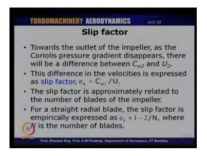
And this difference in the velocities is basically, expressed as a fraction, that is, C w2 by u 2, which is usually denoted by sigma and the sigma is, is a factor of actual blades. It will be less than 1 and one would like to have a slip factor close to 1. So, that means, C w2 will be equal to u 2 and it will lead to much higher, let us say, efficiency and pressure ratios for, for the same rotational speeds and impeller diameter.
