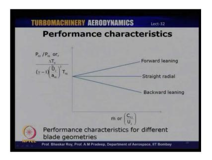
So, if we look at the performance characteristics, either in terms of pressure ratio or the temperature rise versus either mass flow rate or the flow coefficient, a forward leaning blade would have a characteristic, which has positive slope throughout.
