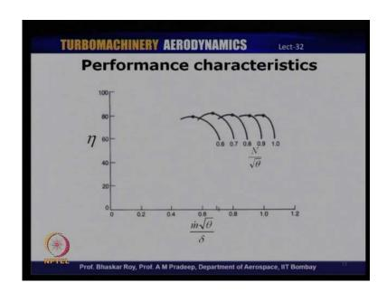
Now, if you look at the efficiency characteristic, again very similar to the axial compressor that we discussed. Efficiency versus mass flow rate for non-dimensional speeds and with increase in speed you can say, that the range of high efficiency becomes narrower.
