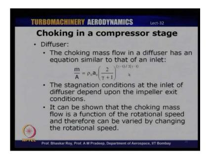
Now, the last component, if the diffuser, the choking mass flow in a diffuser has an expression the same as that of inlet, so it is again a function of the inlet condition for the diffuser. So, mass flow rate is function of rho naught a naught into 2 by gamma plus 1 raise to gamma plus 1 by 2 into gamma minus 1.
