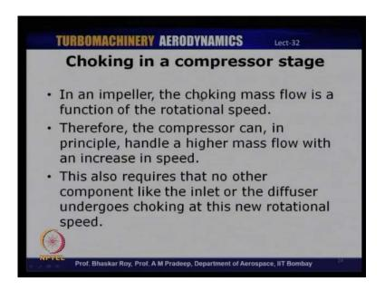
Choking mass flow in an impeller is basically, function of the rotational speed and compressor in principle should be able to handle a higher mass flow with an increasing
