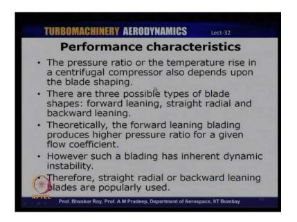
Now, in a centrifugal compressor the pressure ratio or the performance is also a type of function of the, type of blade, that is used in a centrifugal compressor.
