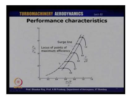
So, if we look at the pressure ratio characteristics versus mass flow rate characteristic, so the previous slide I had shown an idealized curve. Here, we have seen that the curve on the left hand side is not possible and beyond this it chokes. So, the actual performance characteristic is limited between these two points B and E and that is what is shown here by these different lines.
