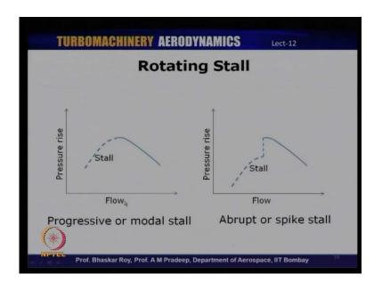
On the graph that you see here on the left hand side, we have pressure rise versus flow. The compressor characteristic operating all the way from choke with decrease in mass flow or as with throttle the compressor leading to higher and higher pressure ratio peak pressure ratio and then the pressure ration begins to drop.
