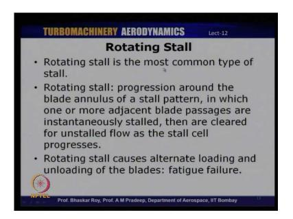
And we will discuss about rotating stall in some more detail and what is meant by rotating stall. So, rotating stall is the most common type of stall that one would encounter in an axial compressor. Rotating stall would basically involve progression around the
