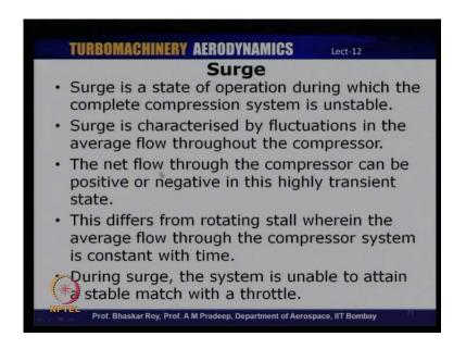
Now, surge is basically characterized by fluctuations in the average flow throughout the compressor, and in this case, the net flow through the compressor can either be positive or negative when its highly transient phenomenon, and this is different from rotating stall where in there is still an average flow which is passing through the compressor and is constant with time, but during surge, this system obviously is unable to attain a stable match with a throttle which is downstream.
