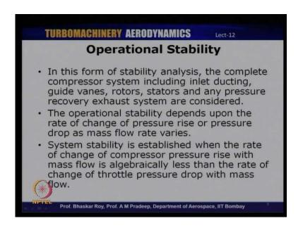
So, in operational stability, the complete compressor system including the inlet ducts, guide winds, the rotor stators of the compressor and the exhaust systems are considered, and operational stability basically depends upon the rate of change of pressure rise or pressure drop as the mass of the rate varies. System stability is established when the rate of change of compressor pressure rise with mass flow is algebraically less than the rate of change of throttle pressure drop with mass flow.
