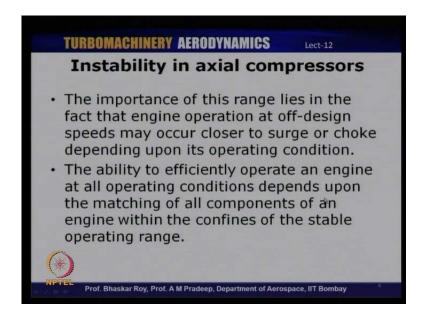
And so, the ability to efficiently operate such an engine at all these operating conditions will also depend upon a successful match of all the components within an engine and also within the stable operating range. So, for example, an engine has, as you has you probably aware and it will typically an air intake, then a fan or a compressor, then the combustion chamber, turbine and a nozzle.
