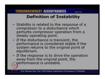
So, stability what in the, in this context of a compressor is basically related to the response of a compressor to a disturbance which perturbs the compressor operation from a steady operating point, and if the disturbance is transient, the performance will be considered stable if the system returns to its original state of equilibrium. If the response is to drive the operation away from the operating or original point, then the operation or performance is unstable.
