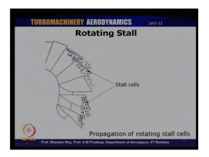
So, as I mention, you could also have more than one set of stalls, stall cells moving along the annulus like you see here, in this example, you have multiple stall cells which are propagating along the tip of the compressor blade. So, you could have multiple number of stall cells. You could have other one stalls cell or you could have number of stall cells, and in fact it has been observed that there are as high as nine stall cells which have been observed experimentally.
