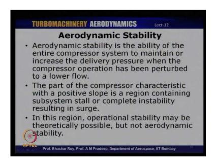
So, this part of the compressor characteristic which has a positive slope is a region containing subsystems stall or complete instability which could lead to surge. So, stall and surge are those two instabilities which we will get initiated if you are to operate on the left hand side of the curve. So, in this region as we have seen, operational stability may still be possible, but aerodynamic stability is not possible.
