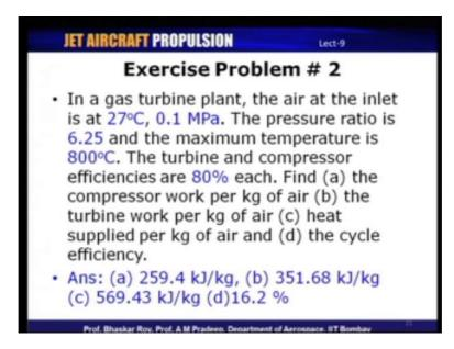
The second problem is in a gas turbine plant, air at the inlet is at 27 degree Celsius and 0.1 MPa, the pressure ratio is 6.25, the maximum temperature is 800 degree Celsius. Compressor and turbine efficiencies are in 80 percent each, find part a, compressor work per kilo gram of air, part b turbine work per k g of air, part c heat supplied per k g of air, and part d the cycle efficiency.
