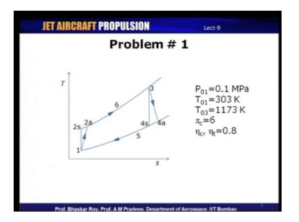
So, here we have a cycle diagram for a Brayton cycle, I have indicated both the actual and the ideal Brayton cycles. So, those points which are indicated with an s, that is 2 s indicates the isentropic point on that cycle, similarly 4 s is for an isentropic process.
