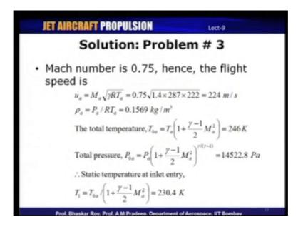
So, Mach number in this case is here given by is given as 0.75 and therefore, we can find these flight speed which is u a, u subscript a is the flight speed which is Mach number times
