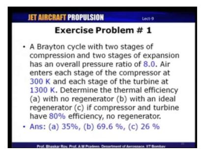
So, you have four different problems as excises a problem, the first one is for a Brayton cycle. So, a Brayton cycle with two stages of compression, when two stages of expansion has an overall pressure ratio of 8.0, air enters each stage of compressor at 300 Kelvin and each stage of the turbine at 1300 Kelvin.
