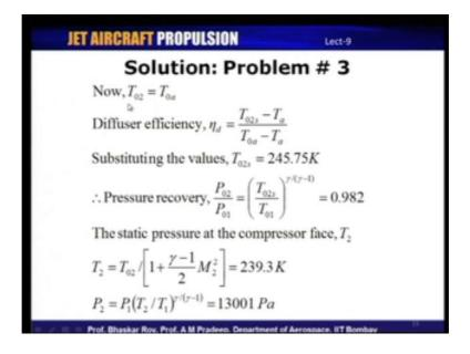
Now, in order to find out the pressure recovery, we will make use of the diffuser efficiency definition. Now, T 0 2 as we know it is equal to T 0 a, and the diffuser efficiency is defined as T 0 2 s minus T a divided by T0 a minus T a, diffuser efficiency is given as 0.95, T 0 a is known you already calculated that, T a is also known.
