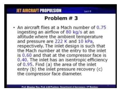
So, the problem number 3 that we have for today is an aircraft flies at a Mach number of 0.75 ingesting an air flow of 80 kilo grams per second at an altitude where the ambient temperature and pressure are 222 Kelvin and 10 kilo Pascals respectively. The inlet design is
