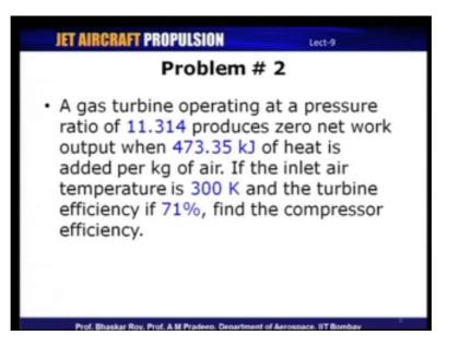
So, let us take a look at what is a second problem that we have for us today, second problem is again a gas turbine problem, again in some sense it is basically a Brayton cycle problem. So, here we have a gas turbine operating at a pressure ratio of 11.314 produces zero net work output when 473.35 kilo joule of heat is added per kilo gram of air. If the inlet air temperature is 300 Kelvin and the turbine efficiency is 71 percent, find the compressor efficiency.
