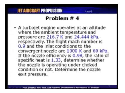
So, the problem statement number 4 is a turbo jet engine operates at an altitude where the ambient temperature and pressure are 216.7 Kelvin and 24.444 four kilo Pascals.
