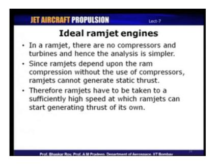
Now, in a Ramjet engine there are no compressors and turbines and therefore, it is analysis is quite simple, because you do not have too many complex geometries present in ramjet and so, Ramjet cannot generate any static thrust basically because Ramjet depend upon ram compression, without the use of compressors.
