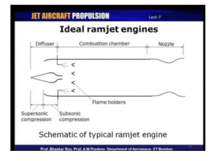
So, let us look at a schematic of a Ramjet I mentioned that it is very simple and it is indeed simple to look at the schematic that, it consists of a diffuser, a combustion chamber and a nozzle.
