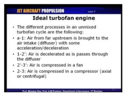
So, the different processes, let us say in an unmixed turbofan will be the following, we have the diffusion taking place between stations a and 2 prime. And then we have compression in the fan between 2 prime to 3 prime compression in the nozzle well compression in the compressor which could be axial or centrifugal is between stations 2 and 3, so 2 to 3 is compression in the compressor.
