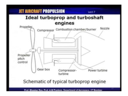
Now this is a schematic of a typical turboprop engine and let us takes a look at what are the different features or components of a turboprop engine, so one of the most prominent components of a turboprop engine is the propeller.
