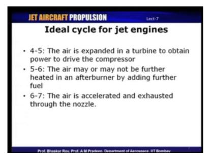
And 4 to 5 is the expansion in the turbine, so the turbine is primarily meant here, in a turbojet engine to drive the compressor; and then, there would be after burning taking place between stations 5 and 6 and 6 to 7 is acceleration and exhaust of the products through in nozzle, so 6 to 7 is in nozzle process in the Brayton cycle or the turbojet cycle.
