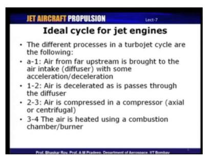
Now, how does this look like in T S diagram we will see that little later, basically the components each of these components have a certain role to play in the whole Brayton cycle. And for example, the diffuser is part of the compression process as we know in a Brayton cycle; there are four distinct processes, the compression process, a heat addition process at constant pressure, then expansion process and again a heat rejection process.
