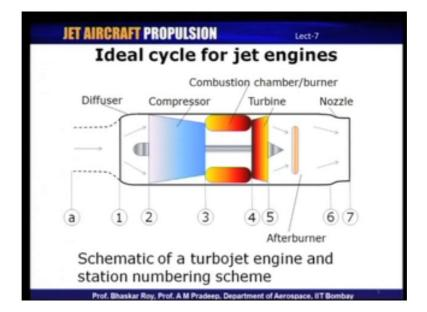
So, here is a schematic of a turbojet engine typical turbojet engine and the different components of a turbojet engines are also shown here. Now, the first component of a turbojet engine is known as a diffuser; diffuser is a component which decelerates the air to velocities, which are suitable for that operation of a compressor.
