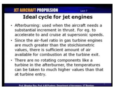
So, turbojet engine with afterburning closely resembles a Brayton cycle with reheat, will take a look at the turbojet with afterburning or reheat as well. And so, basically afterburning is something, which is used when they in an aircraft needs substantial increment in thrust for example, when it has to accelerate and cruise at a supersonic speeds.
