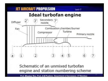
So, this is one schematic, that I have of a turbofan engine this is basically an unmixed turbofan engine, I will explain what is unmixed shortly. And you can see that the fundamental difference between this engine, which is shown unmixed turbofan and pure turbojet is the first component that you can see here, well rather the second component that is a fan.
