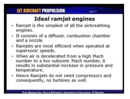
So, Ramjet are suppose to be most efficient only when they are operated supersonic speeds and the basic principle behind the ramjet is that, when air is decelerated from a very high Mach number to very low subsonic Mach numbers, it results in substantial increase in pressure and temperature.
