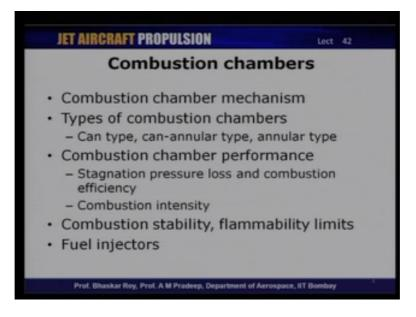
And, after we discussed about the rotating components, we then took up the non-rotating components. And so, we started off with the combustion chamber. That is one of the non rotating components. So, combustion chamber is the heat adhesion unit of... If we look at the Brayton cycle, there is one process which involves heat adhesion. So, combustion chamber is the part of that Brayton cycle, where heat adhesion takes place. we have seen the mechanism of combustion chamber itself.
