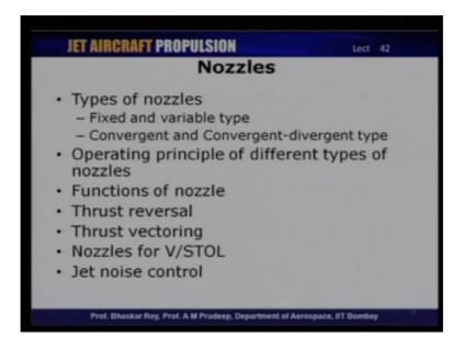
So, after intakes with the other component that we had for discussion, the last component of a jet engine, that is the nozzle. So, similar to intakes we also classified the nozzles in different types. We could have fixed nozzles, a variable type nozzles; one may have the conversion type of nozzle, convergent-divergent type nozzles.
