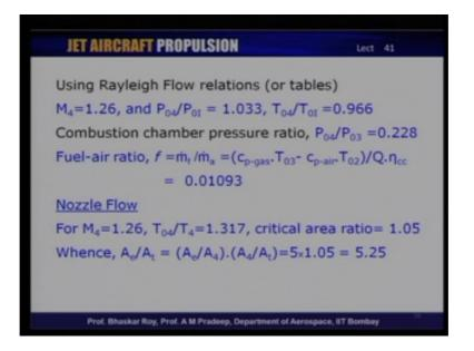
So, using those we can get the parameters across the combustion chamber. So, let us do that across the combustion chamber. So, the entry Mach number that we have found is from the shock relations most 3.3. The moment you have a burning of the fuel the Mach number reduces to 1.26 because the temperature is now very high and so, even if the flow velocity
