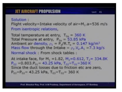
Let us look at the solution that we can find prescribed is that the flight velocity is for that Mach number would be 536 meters per second; that is at Mach 1.818 at the prescribed altitude. And the total temperature at the entry would be T 0 a, that will be 360k; and total pressure at entry P 0 a would be 53.85 kilo Pascal.
