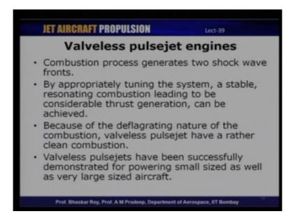
So, in this combustion product process it generates to shock waves and by appropriately tuning the system adjusting the length of the system, one can achieve a stable resonating combustion which leads to considerable thrust generation.
