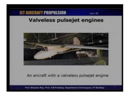
So, this is one example one picture of an aircraft a French aircraft, which has actually got a Lockwood Hiller type of a valve less pulsejet. You can see the engine here this is the valve less pulsejet engine where you can see the u bend and the long exhaust pipe. So, valve less pulsejet engines are characterized by a rather long exhaust pipes you can see the long exhaust pipe here. So, this is one example of an aircraft, which had valve less pulsejet engine.
