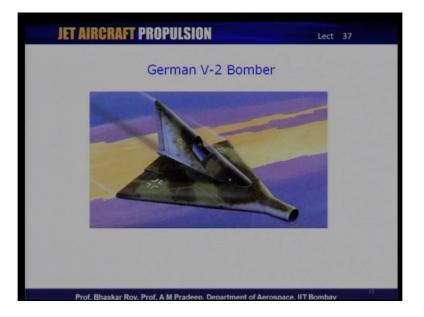
This is a the German V-2 Bomber in which ramjet engine was a utilized and as you can see here, it is a very simple aircraft in which the flow came in right from the nose and indeed this was not a supersonic aircraft; it was actually a subsonic aircraft.
