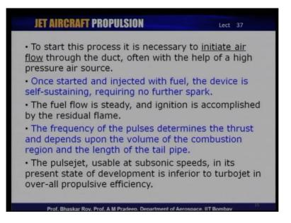
So, let us take a look at a little more details about how the pulse jet engines operate. To start the pulsejet engine, it is necessary to initiate air flow through the duct often with the help of a high pressure air source. Now, this is what is necessary to be done, because the pulsejet engine does not come in with a ram effect. It does not come in with a high pressure and to initiate the flow through the duct; it is often necessary to create a flow, because there is no flow to begin with.
