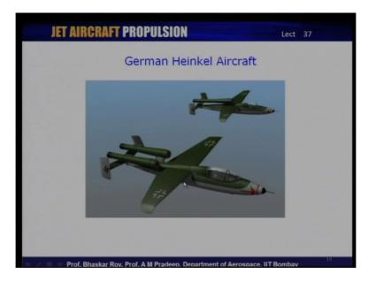
This is the kind of a German Heinkel aircraft, which use the pulse jet engine during the world war. They used it quite successfully for flying of the aircraft it was indeed a very successful a deployment of pulsejet engine for an aircraft flight.
