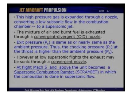
The high pressure grass which is been created through the combustion process the pressurization was done by the intake process and the combustion created the gas. Now, this high pressure, high temperature gas is now expanded through a nozzle, which essentially converts a low subsonic flow in the combustion chamber or coming from the combustion
