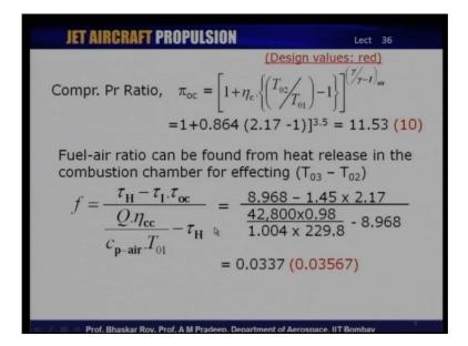
This means that the compression ratio the pressure ratio across the compressor would indeed also be more than the design point pressure ratio which was prescribed as 10 and we see here that the off design point we have a pressure ratio which is 11.53 using the simple thermodynamic relations that we have done before probably more than once. Now this means that in terms of the compression ratio we are now getting more
