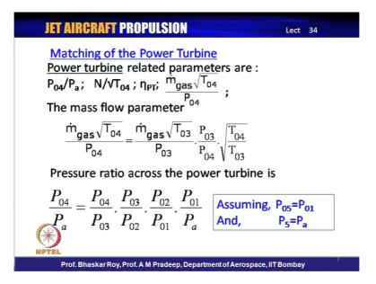
Now, power turbine or free turbine as it is of use we use the word power turbine, because it is often used for powering the a fan or the propeller, which often is used in a two spool engine, which means the power turbine, and whatever it is powering that is fan or propeller is on a separate shaft, which is a power shaft and this needs to be matched again separately; other than the core generator ma or the gas generator matching that we have done just now.
