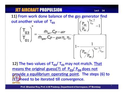
On the other hand, if you do the work balance between the gas generator components of compressor, and turbine if you write down the mass work done using the mass flow of the air, and the gas that is compressor and turbine, and the operating efficiency is the compressor and turbine and the pressure ratios valid across the compressor and that valid across the turbine. And if you again put them together you get T 0 3 by T 0 1. Now, this could possibly be
