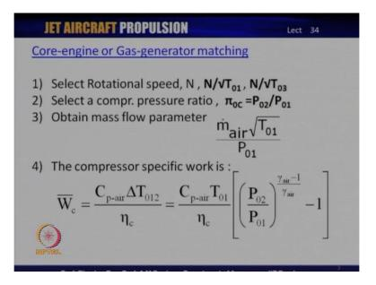
The core engine is quite often also referred to as the gas generator simply, because it also produces the hot gas which of course, runs the engine, and hence quite often many people refer to its simply as a gas generator. Now the core engine as we know is composed of the HP compressor, and the HP turbine and some are between them there is a combustion chamber.
