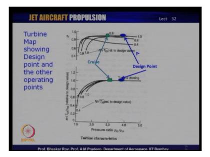
Let us take a look at the turbine which is one of the important components. The design point typically operates at certain condition, where the turbine is likely to be chocked and this is where, you have a very good efficiency. And it is in the modern aircraft design, you could have the cruise operation which is far away from the design and it is entirely possible that at
