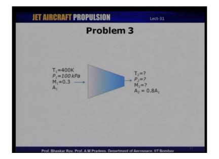
So, this is the problem statement. We have a convergent nozzle, inlet static temperature, static pressure and the Mach number are specified and the exit area is given as 0.8 times the inlet area. We are required to find out the exit static temperature pressure and the Mach number.
