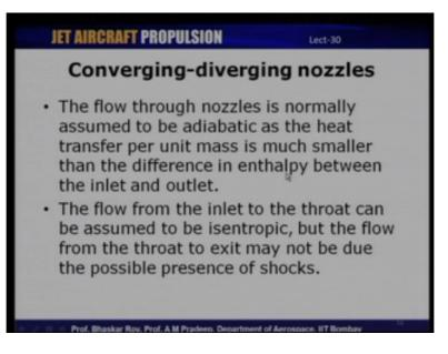
So, what we will do is we are going to assume as we have done for convergent nozzle that the flow is adiabatic because heat transfer per unit mass is much smaller than the difference in enthalpy between inlet and outlet. The flow can be assumed to be isentropic up to the throat. But from the throat to the exit, it may not really the isentropic; because there could be possible shocks especially under certain operating conditions.
