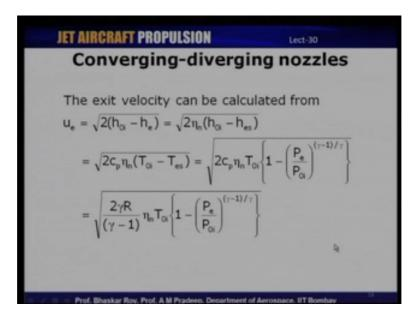
So, the exit velocity; So, which we have also derived for the cycle analysis is u e which is square root of 2 in to h naught i minus h e, which in terms of efficiency becomes 2 in to eta n in to h naught i minus h e s and this again in terms of temperature is 2 c p eta n in to T naught i minus T e s. This is on simplification 2 gamma R by gamma minus 1 in to eta n in to T 0 i multiplied by 1 minus P e by P 0 i raise to gamma minus 1 by gamma.
