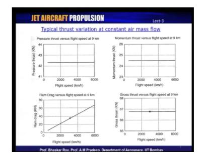
Let us take a look at simple thrust variation characteristics of a simple jet engine that we looked at. Let us say, a constant air mass flow. Supposing the air mass flow through the engine is held constant, let us say by some design of the intake. So, at a particular altitude, in this case we are looking at a flight at an altitude of 9 kilometers which is quite often a normal altitude at which many of the jet engines actually fly with aircraft.
