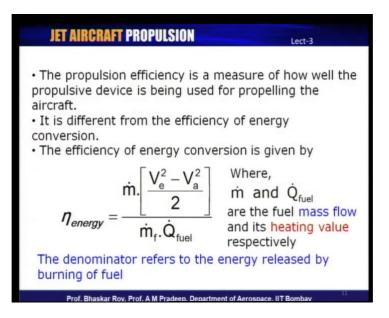
The propulsive efficiency that we are looking at that we have just defined is actually comparable let us say to a propeller efficiency, where propeller is the propulsive device and when we have a propeller driven engine, the propulsive efficiency of a typical jet engine would be comparable to the propeller efficiency of the propeller driven engine or propeller driven thrust making device.
