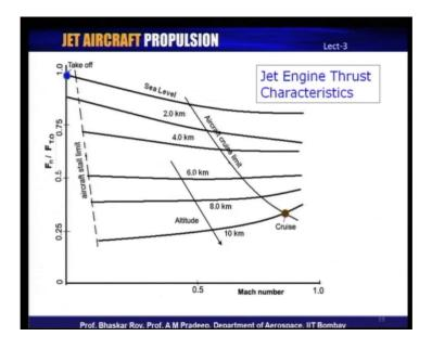
Let us take a look at the overall thrust characteristics of a typical jet engine and as we see here the thrust characteristics have been computed typically for at various altitudes starting with sea level, then 2 kilometers and going all the way up to 10 kilometers which is often a good cruise altitude for many of the aircraft that are flying around.
