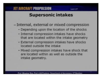
The other type of classification is depending upon the location of the shock itself, it could be either internal compression, could be external compression or a mixed compression intake. In internal compression intakes the shock are located within the intake geometry itself that is you have shocks, which are inside the intake geometry which cause deceleration supersonic to subsonic and then the subsonic diffuser which decelerates high subsonic to low subsonic.
