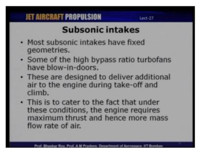
So, in the case of intakes most of the subsonic intakes as I mentioned have fixed geometric except in certain cases where we may use blow in doors used in high bypass turbo fan engines, which basically are meant to deliver additional mass flow rate to the air engine during takeoff and climb.
