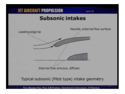
So, a typical pitot intake as I mentioned is usually axis symmetric because of the like the intake which I had shown for the transport aircraft that is axis symmetric pitot intake.
