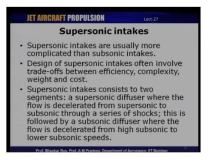
So, supersonic intakes are usually it is a fact that supersonic intakes are usually more complicated than subsonic intakes and the design of these intakes usually involve tradeoff between efficiency complexity weight and cost and the that is something that the designer would have to eventually optimize and try to develop a design which will involve some sort of tradeoff between all these parameters. And supersonic intakes will usually consist of two components of or two segments.
