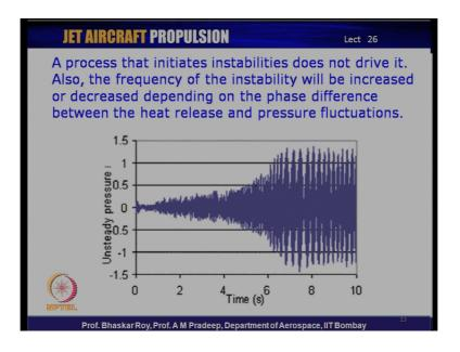
So, will look at some of the combustion instabilities that can occur the if you see here the combustion that is initiated from here and after very small amount of time, you can see it develops into instability and the frequency of the instability can get the decreased or increased depending on the phase difference between the heat released and the pressure
