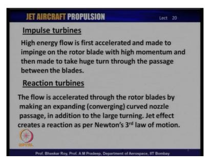
Hence, we have two kinds of turbines: the impulse turbines, in which the high energy flow is accelerated and made to impinge on the rotor blade with initially high momentum and then it takes a huge turn through the passages which are created between the blades. The aero foils create the passage and then we the impulse action; the reaction turbines on the other hand not only take a huge turn but, in addition they execute a large acceleration through this converging curved nozzle.
