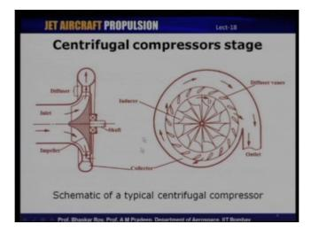
A centrifugal compressor is it looks entirely different as compared to axial compressors. Let us take a look at what they look like, so what I have shown here is a typical a centrifugal compressor just a schematic of one of them, so there are numerous designs of centrifugal compressors, this is just one of them. And there are two views of the same compressor that I have shown one is the side view and this is the front view.
