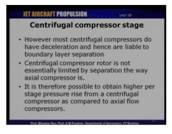
So, with no change in relative velocities it means that centrifugal compressors are not really subject to issues of flow separation, but most of the modern day centrifugal compressors also have certain amount of deceleration taking place. And which means that there are also liable to separation in some sense or the other.
