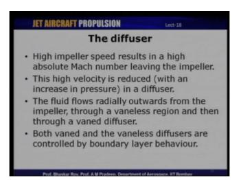
So, diffuser is a component, where in which is similar to a stator in an axial compressor in axial compressor as we know, we consists of a rotor followed by a stator. The diffuser has more or less the same function in centrifugal compressor and in a diffuser the other aspect is that if we at the periphery or a exit of the impeller usually we have a very high velocity and therefore, it might lead to very high mach numbers, which leave the impeller.
