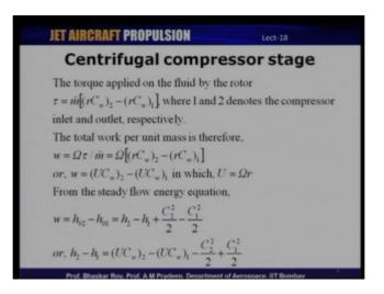
So, the first thing that we will do is to relate the enthalpy raise across a centrifugal compressor to the geometric and velocity parameters. So we know that the torque that is required to generate the pressure ratio or the torque applied by the rotor on the fluid is a function of the mass flow rate, and the difference in the tangential velocity.
