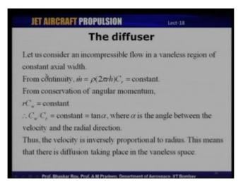
And so, if you look at for an incompressible flow at least the mass flow rate is basically density times the cross sectional area times the radial velocity, which is a constant and if we have to have if we look at the conservation of angular momentum then we have r times C omega, which is a C w; which is the tangential velocity is a constant that is from conservation of angular momentum.
