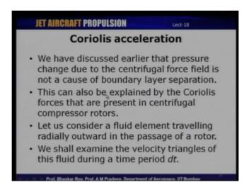
So, we will try to get some elementary idea of what this coriolis acceleration means and what it does to the performance of centrifugal compressor rotors. So in the case of centrifugal compressor rotor the pressure change in the case of centrifugal compressor rotors, the risk of boundary layer separation is probably lower than that of axial compressors because a pressure raise is primarily because of the centrifugal force field and not really because of the deceleration of flow.
