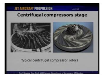
So, this is a schematic. I will now show you two typical centrifugal compressor rotor photographs of two different types of centrifugal compressors. So these are two centrifugal compressor rotors, one of them is a very old generation design of a centrifugal compressor, this is inducer as I had just discussed, and these are the impeller vanes; you can see that these vanes are straight
