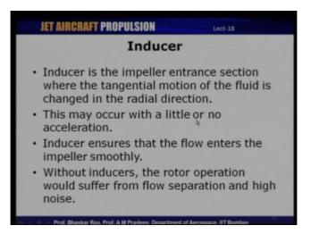
Now, the other component now impeller is as I said the main component heart of a centrifugal compressor that is the rotor, the other component that is of interest to us is the initial part of the impeller that is known as an inducer I have already shown you some pictures of the inducer. Inducer is the initial part of an impeller, wherein the flow is guided smoothly into the impeller because I mentioned that the axial flow which is entering into the compressor becomes radial through the impeller.
