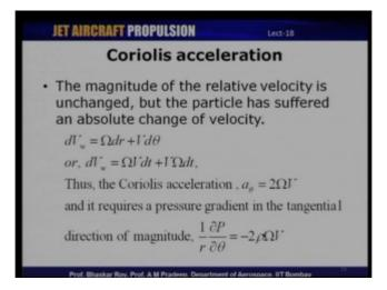
So, this velocity, which if we are assuming that the magnitude of relative velocity remains unchanged there is a slight change in the absolute velocity, which the particle undergoes that is basically given by this component that is d C, so this is assuming that relative velocity does not change much, which is what is clear from this velocity triangle we are not changing relative velocity much, but it does it definitely leads to a change in the absolute velocity.
