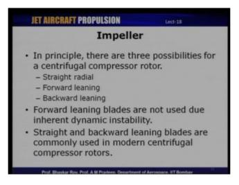
So, what we will discuss next is about one of the components of a centrifugal compressor. When I showed you the schematic, you had seen that there are different components of a centrifugal compressor. We have inlet duct then there is an impeller. And one constituent of an impeller is inducer, which I will discuss a little later. Impeller is the main section of a diffuser of a centrifugal compressor. It is a rotor of a centrifugal compressor.
