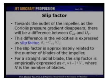
So, because of the presence of the coriolis acceleration we have seen there is a tangential variation in velocity and so, if **if** you were to look at the velocity triangles at the exit of the impeller, this variation is going to effect the velocity triangles at the exit, now that is as the fluid element lives the impeller there is going to be a slight variation in velocity triangles from what it should have been as per our earlier analysis.
