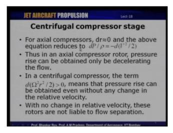
So, let us look at that equation once again. So we have d P by rho is d omega square r square by 2 minus d V square by 2 for an axial compressor, the radius change of radius is 0, because we consider for the same mean diameter or any other circumferential location.
