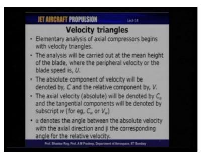
So, what we do is that we will carry out or the analysis that we are going to do is limited to a certain height of the blade. We will take the main height of the blade, and we will assign the blade speed or the peripheral velocity to a symbol U. So U denotes the peripheral velocity or the blade speed at that particular station, at which the analysis is carried out. And we are going to carry out this analysis for the main blade height.
