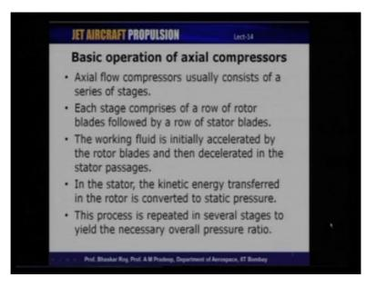
So, axial compressors form one of the basic components or aspects of a gas turbine engine, and in axial compressors as you might have already noticed that they usually consist of a series of stages, and each stage basically comprises or consists of a row of rotor blades followed by a row of stator blades.
