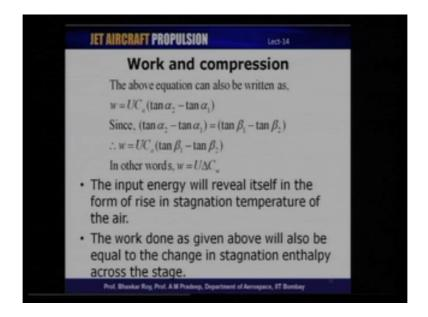
So, if you were to look at the first equation we wrote it was U by C a is equal to tan alpha 1 plus tan beta 1 and U by C a is also equal to tan alpha 2 plus tan beta 2. We combine that with this worked on equation, then we get work done per unit mass is equal to U times C a into tan alpha 2 minus tan alpha 1.
