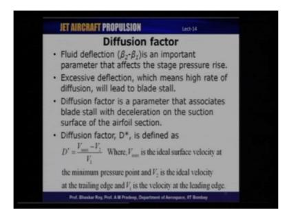
So, fluid deflection is a basically what decides the pressure ratio one of the parameters which decides the pressure ratio but, there are certain limitations to that. So, diffusion factor is a parameter that associates the blade stall with deceleration on the section surface of the airflow. So, it's basically defined as the difference between the maximum velocity, and the minimum velocity that is at the trailing edge to the inlet velocity at the leading edge. So V
