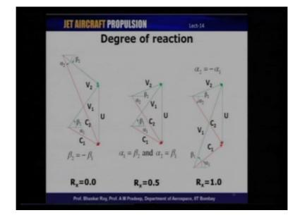
So, the velocity triangles would look something like this for all these three cases if degree of reaction was 0 then we get beta 2 is minus beta 1. So, this is beta 2 here this is exactly opposite equal and exactly opposite to that of beta 1; this is how it would be if we have an impulse balding for an axial compressor degree of reaction equal to 0.5 means alpha 1 is equal to beta 2, and alpha 2 is equal to beta 1, so that is the velocity triangles are mirror images of one and other.
