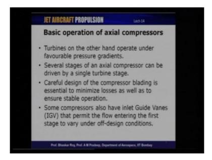
So, on the other hand turbines do not really have this problem, turbines always operate in a favorable pressure gradient mode and therefore, it is possible to have a much larger pressure
