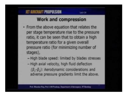
So, what we can see that the it basically the equation relates the temperature raise per stage to the pressure ratio, and so to obtain a high temperature ratio for a given pressure ratio that is to basically minimize the number of stages. We could either increase the blade speed or axial velocity or fluid deflection but, increasing the blade speed has certain limitations that is if we if we were to rotate the blades at very high speeds it can obviously lead to very large amounts of stress.
