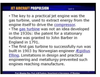
You see the key to a practical jet engine was the gas turbine from which it indeed derives its name. The basic jet engine is technically also referred to as a gas turbine engine; and the key to this is actually the operation of a turbine or gas turbine, which is used to extract energy from the engine itself; and you will need this gas turbine to drive a compressor.
