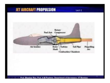
If for example, if you put such a engine inside the body of the aircraft this is the scenario, you would probably have with you the engine is good in proper buried inside the body of an aircraft; and air has to be ingested into this engine; so, you would need rather long air intake system; we will be talking about the intake system later on in this course.
