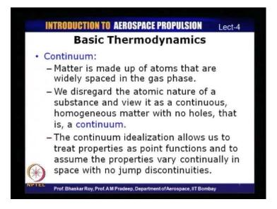
The other principle or the assumption that we are going to make is known as continuum. Continuum refers to the continuity within a system. I will explain that shortly. As we are all aware, matter is made up of atoms, which are widely spaced especially when it comes to the gaseous phase. In classical thermodynamics, we would want to disregard the atomic nature of a substance and view it as a continuous, homogeneous matter with no holes or void, that is, it is a continuum.
