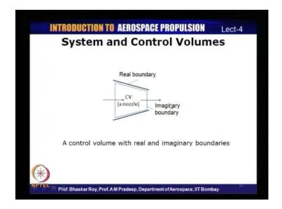
Yet another example: here we have an example of a control volume, which is an open system, which has both real as well as imaginary boundaries. The example that is shown here is that of a nozzle. A nozzle is a section, which is again very often used in engineering systems and is a system, which is used for accelerating a flow in a subsonic mach number flow.
