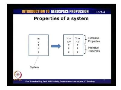
Now, let us look at an example, which will help us in explaining what are intensive and extensive properties. What is shown here in this example is a system, which has different properties, which have been defined here in terms of its mass, volume, temperature, pressure, density, etcetera. If we were to split the system exactly into half like what is shown here on the right hand side, we have a splitter, which splits the system exactly in to half.
