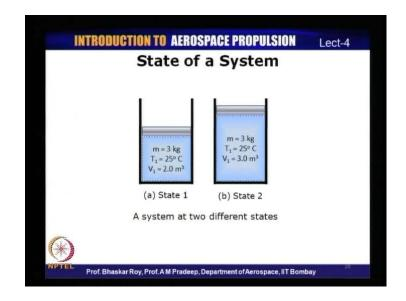
Let us look at an example, which will help us in understanding this. Here we have the piston-cylinder example again. On the left hand side, we have the system which has let us say - a mass of about 3 kgs, temperature of 25 degree Celsius, a volume of 2 meter cube. This defines the state of this particular system at particular instant of time.
