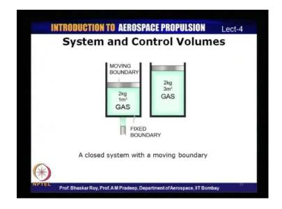
Let us look at one example of a closed system, which has a movable boundary. What you see here is a closed system. It is a closed system because there can be only energy transfer across the system boundaries. There is no mass transfer across the system boundaries and therefore, it is a closed system.
