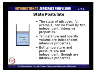
The example that is shown in the slide is that of nitrogen, which is again host with in a piston-cylinder assembly. We can see that the state of nitrogen for example, can be fixed by two independent, intensive properties as per the state postulate. Here we have defined
