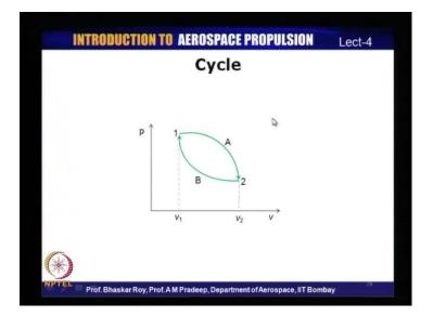
If the same example - we had the process, which is coming back to its initial state, then this is referred to as a cycle. For example, if this piston-cylinder assembly was initially at station 1, after the whole process, it has come back. That is, after an expansion; that is, reduction in volume, increase in volume, and reduction in pressure. Then, further it is compressed back to its initial state. This is referred to as a cycle. That is, the initial state and the final state are identical.
