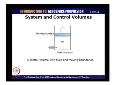
Let us look at an example, which combines the previous example as well as this example in some sense because you have an open system here with a moving boundary. We had already seen an example of an open system, which has real and imaginary boundaries. Here we have an example, which has often open system that is a control volume, which has both fixed boundary as well as a moving boundary.
