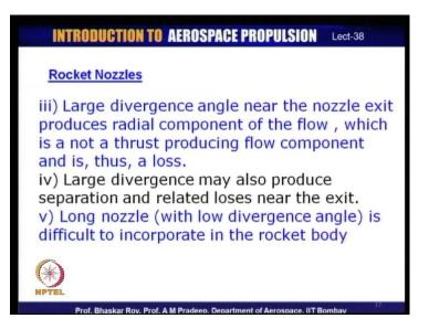
So, the large divergence angle is not exactly a very preferred nozzle shape. The large divergent has another issue and that is the flow under certain cases of over expansion. When it reaches very close to over expansion could produce separation and the separation would immediately create loses near the exit.
