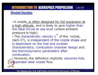
On the other hand, if the nozzle is design for a full expansion which it is often at high altitude, it is likely to give higher than ideal thrust at sea level, where the ambient pressure is actually on the higher side. So, you could have an ideal thrust calculated at sea level, but you could end up actually giving getting more thrust than you have calculated at the beginning. If it is design in such a manner, that the full expansion is actually at high altitude and it is often designed that way.
