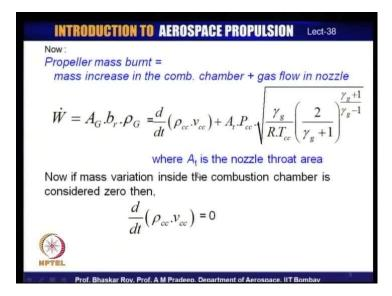
Now, the propellant mass that is burnt there the usage of the mass and that is what that comes out from the nozzle for creation of thrust. That can be given in terms of normally we are giving in terms of weight flow and that is normally the mass increase in the combustion chamber. That is the mass that is burnt from the grain and the gas flow that is happening through the nozzle.
