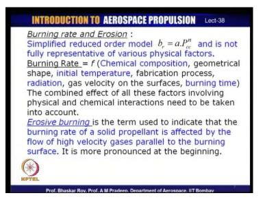
Now, the burning rate that we are talking about and we have written down simply in terms of b r equals to a into P cc to the power n. Now, this is a simplified expression. A simple way of mathematically catching the burning rate and gives us a first cut notion about what the burning rate could possibly be. In engineering, one always likes to have a number, a calculated number which gives us some idea about what is happening.
