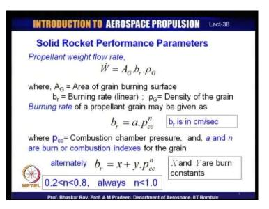
So, if we can now move on to some of the solid rocket performance parameters, if we look at the fundamental issues that we have discussed before, one is that that the rocket always uses propellant use in terms of weight flow. And if we use that, we get a weight flow of w dot which is as usual as for continuity condition is decided by the grain area of the burning surface. The rate of burning and the density of the grain at which, it is being housed inside the combustion chamber.
