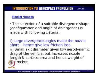
The selection of this divergent shape is can be made of certain simple criteria and we will write down here some of the simpler criteria that needs to be followed. You see the large divergence angle makes the nozzle very short, and hence, it gives very low friction loss.
