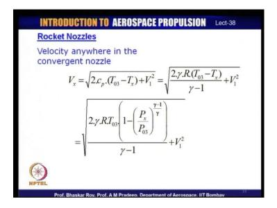
The velocity anywhere in the convergent nozzle can then be given by simple again isentropic flow relations and you could get them in terms of the basic parameters of pressure at any point which is P x and pressure coming from the entry to the rocket nozzle P 0 3 and then the gas values - T 0 3 and R and gamma. So, these things give you the velocity anywhere in the convergent nozzle.
