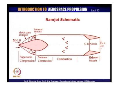
C-D nozzle is used normally when ideally pressure ratio available that is, total to static pressure ratio available is of the order of at least 2. So, normally you would use it only when the pressure ratio is of the order of 4 or 5 and that is the kind of pressure, which is normally generated and as a result of which, this C-D nozzle now creates a supersonic exhaust jet.
