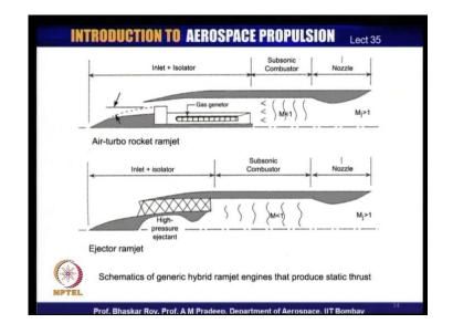
Let us go back just for a minute. This isolator actually is a part of the ramjet and it is called isolator because it is a supersonic isolator, which allows a long train of shocks before the flow is delivered into the combustion chamber. It also isolates the combustion chamber from the intake ambient pressure or temperature changes, which happens with the change of altitude. So, this is often called an isolator because it houses a long train of shocks.
