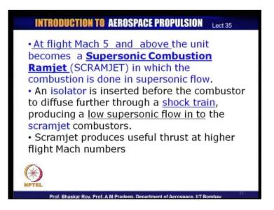
At Mach 5 and above, the normal ramjet cannot diffuse the flow any further to subsonic values for combustion purpose. As we were just discussing that, if you have intake for high supersonic flights, those intakes are full of shocks and as we have just seen, they are full of shock trains. So, the flow is coming through a large number of shocks - maybe 8, 10, 15 shocks, which are inside the intake system which includes an isolator.
