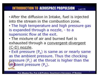
Some of these are the features. The fuel that is injected into the stream is after the diffusion of the flow through the intake system through supersonic and subsonic compression and once the air has been sufficiently compressed and sufficiently diffused to low velocity, the fuel is injected. As a result of which, we get a high temperature, high pressure gas available from the combustion chamber and this gas is what is then released through the nozzle.
