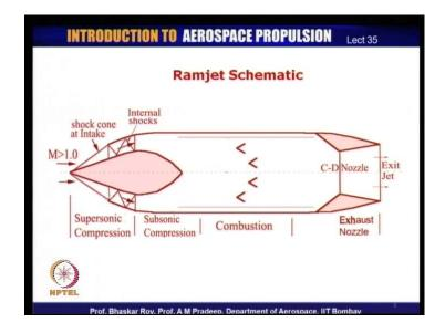
If you look at the ramjet schematic, you would see that there is a flow coming from the intake side, which is at Mach number normally greater than 1, quite often the modern usage is Mach number would be pretty close to 5 or even higher. Some of the ramjets or scramjets being used would be at flying Mach order of the order of 8, 9 or 10.
