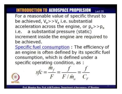
What we see now from these equations which have been derived from fundamental principles that the reasonable positive specific thrust to be achieved V e needs to be somewhat higher than V a.
