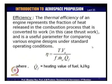
The efficiency of the engine also can be calculated as per basic definition of efficiency which is normally the thrust work that is created by the jet engine, divided by the fuel energy that has been put inside the combustion chamber in terms of basic fuel energy or heat energy.
