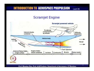
We can look at a Scramjet engine and indeed, a Scramjet powered vehicle over here, as you can see, the flow is coming through the intake system and then let us say this part is a vehicle body and this is your jet engine and outside the jet engine itself, you have a vehicle body, which is angled over here and it is often called the external ramp intake.
