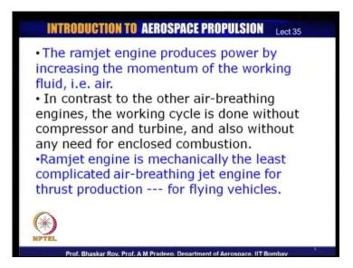
If we look at what are the key features of a typical ramjet engine, firstly, it produces power by increasing the momentum of the working fluid, which in our case is the atmospheric air that is available.
