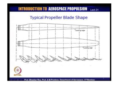
Let us quickly go back to the propeller diagram which we have looked at right in the beginning. You see all these blade shapes need to be created by design. The aerofoils need to be set at various designations, but quite often one starts off with one of the blade shapes which could be somewhere around here, which is to begin with representative of the entire propeller.
