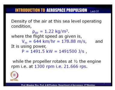
Let us see how the solution of this problem would proceed. The density of the air at this operating condition that is a normal sea level and that is rho air as given as 1.22kg per meter cube; that is the standard air density at sea level and the flight speed is given as 644 kilometers per hour which translates to 178.88 meters per second.
