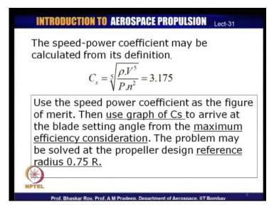
So, propeller reference radius is often chosen during the design and we are going to solve our problem at that reference radius, which is as I mentioned representative essentially of the entire propeller actually. So, we will proceed along those lines.
