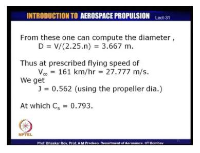
Let us proceed along this. From this, we can now compute that the diameter of this propeller based on these parameters would be 3.667 meters, and as a result of which, we get a value of J now. The velocity, forward velocity we had already calculated 27.77 meters per second as the alternative flying speed that was specified in the problem.
