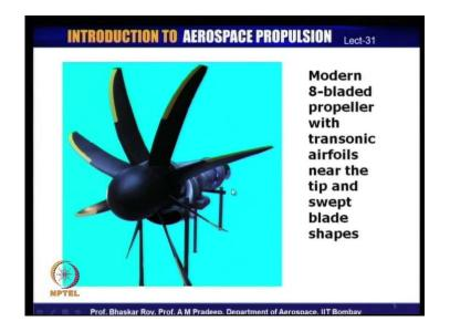
We can look at a typical modern propeller as you can see here, it is made up of eight propellers and each of these propeller is made up of a large number of aerofoil shapes and some of the aerofoil shapes towards the tip of the propeller are very likely to be transonic aerofoils.
