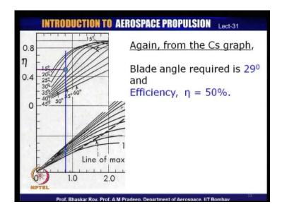
Now, you can use this value of advance ratio and this value of speed power coefficient to find a new solution and we use the graph again. What we see here that, we are now at a rather low speed power coefficient, a low flying condition, and at which, the advance ratio is also rather low and our solution point is somewhere over here.
