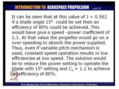
So, what can be done is - if you now set the blade setting at 15 degree, you could actually get an efficiency of 80 percent. Now, this is possible with this propeller only, and the
