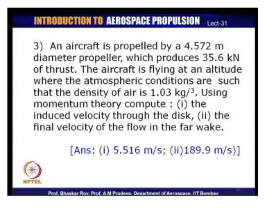
The third problem is an aircraft is propelled by 4.572 meter diameter propeller, which produces 35.6 kilo Newton's of thrust. A thrust as we see now would be expressed in terms of kilo Newton's for most of the aircraft engines, including propellers and all jet engines.
