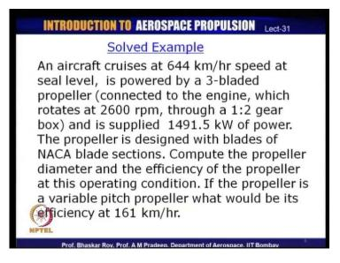
Now, before I give you the problems, I will try to solve a problem for you and this problem is of a variable pitch propeller and this propeller is a little more conventional propeller. What it states here is - it is used in an aircraft which is cruising at 644 kilometers per hour at sea level to begin with and is powered by 3-bladed propeller.
