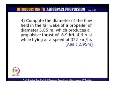
The fourth problem is the compute the diameter of the flow field in the far wake of a propeller of a diameter 3.05; that means the propeller has a diameter of 3.05 and it is producing a thrust of 8.9 kilo Newton's while flying at a speed of 322 kilometers per hour. What would be the diameter of the flow field in the far wake of a propeller? So, that is the problem statement which is given here should be able to find from the propeller theories that we have done.
