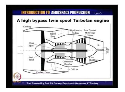
Some of these things, we will probably talk about more and more as we go along. The next kind of engine that we are looking at is high bypass engine as we have seen from the propulsive efficiency concept that the higher the bypass flow, higher the mass of activation, more is the propulsive efficiency.
