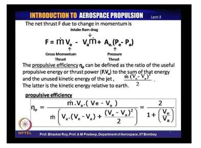
However, if that happens from the earlier equation over here assuming that this pressure thrust is 0 the trust produced actually be pretty close to 0; that means when the propulsive efficiency is 100 percent the thrust produced would be 0 obviously, such an engine is of no use to us. The solution is that if you have very small change in the velocity, which operates on a very high mass flow, then a substantial amount of thrust can be produced.
