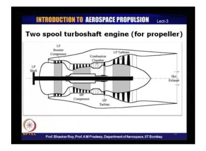
This is a kind of engine that is used normally in flying helicopters and these are called turbo shaft engine; this typical two spool turbo shaft engine these are used for running the propellers or the routers of an helicopter.
