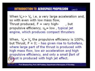
We shall see later on that this propulsive efficiency does have an impact on the fuel efficiency that everybody is so concerned with. The other end of the picture is supposing, when the exit velocity is equal to all let us say, almost equal to the entry velocity V a then, the definition tells us that numerator will be equal to the denominator both would be 2 and as a result of which your propulsive efficiency is actually going to be 100 percent or very close to 100 percent.
