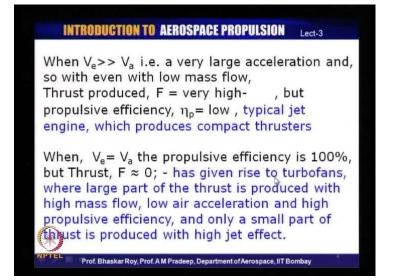
Now, the fall out of this very simple propulsive efficiency definition actually tells us of few stories. Let us see, what actually can be extracted from this very simple definition of propulsive efficiency. For example, your exit velocity is rather large compare to the entry velocity of the air that means a very large change of velocity or a large amount of acceleration as occurred through the propulsive device and quite often that happens with a rather low mass flow.
