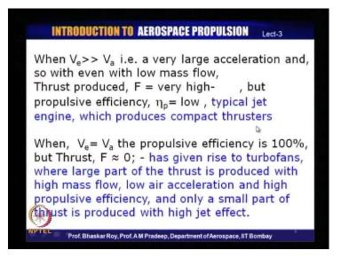
You could get a reasonably good amount of thrust produced but in such a case the propulsive efficiency is going to be low because this ratio is now rather big. The denominator here is going to be much higher than the numerator which is 2 and the propulsive efficiency thus would come out to be somewhat on the lower value. This is typical of a jet engine in which normally a large exhaust velocity is observed.
