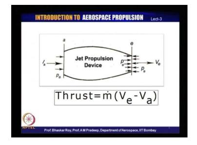
The basic concept of jet propulsion comes from the simple concept or an idea that if you have a device in which a certain amount of working fluid and in our case this working fluid is almost, invariably air. As a result of which, all jet propulsion devices that we are talking about are essentially air breathing engines. These air breathing engines have propulsive method by which this is illustrated in this picture.
