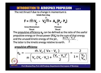
Let us now, look at the equation that we were talking about; the thrust equation we had seen the first part which constituted what we had called the momentum thrust. The first part of the momentum thrust can be called the grass momentum thrust, which is the reaction principle at the exit of the propulsive device of the engine. This is normally the component, which is produced by the incoming flow and this is often referred to as the intake ram drag.
