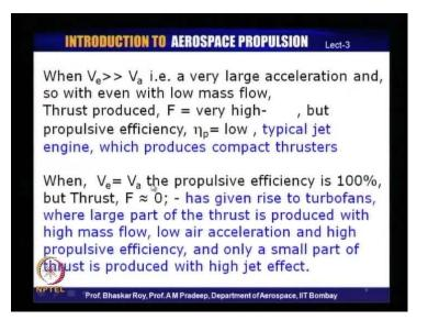
So, we now turn our attention to the mass flow and not the change of velocity. If we can have a propulsive device when the operative mass flow is very high in such a case, you can produce a requisite amount of thrust, a substantial amount of thrust, and that trust production mind you, now is going to be with very high propulsive efficiency.
