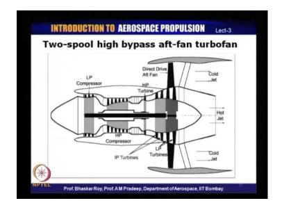
This is an aft fan in which the fan is at the rear, which is mounted actually on the turbines. So, the turbines are directly running the fan, you do not have a shaft here and as a result of which the transmission efficiency here is almost 100 percent there is no shaft. This is a two spool arrangement this is virtually the third shaft or third spool, which are running independently of these two spools.
