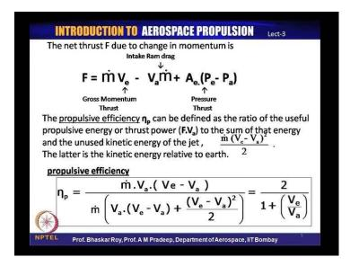
Now, the engine designer has to be very careful in designing the nozzle to ensure that under no operating condition the exit pressure P e should be less than the atmospheric pressure P a, because if that happens we are going to have a negative component over here and we are actually going to get a negative thrust.
