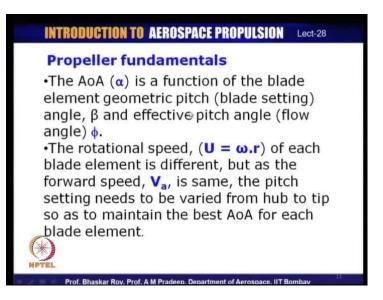
Whereas, in this case, for the root, the angle of attack also needs to be kept within in a certain value, but the value of phi here is going to be high. As a result of which, your blade needs to be given a twist. This is from the fundamental fact that the rotational speed omega is constant from root to tip, but the actual rotational speed that is U varies from root to tip - the tangential velocity varies from root to tip for each element of the blade.
