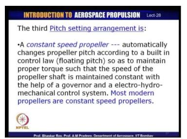
However, the most modern kind of pitch setting is referred to as constant speed propeller, which is often controlled by a control mechanism. The propeller pitch has a built-in control law, which is often also referred to as floating pitch. So, have to maintain torque balance between what the propeller needs at a particular time of operation and what the engine is supplying. This torque balance is extremely important during the entire operation of the propeller.
