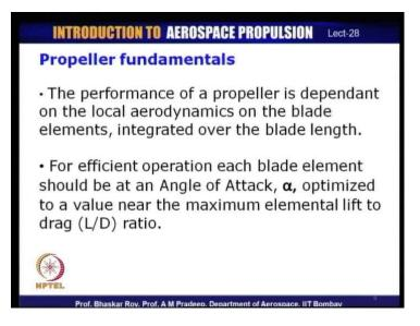
For efficient operation of each of these blade elements, which are airfoils, as we have seen, we need to create an appropriate angle of attack. As we know, all airfoils have a characterized value of angle of attack, at which, it is most efficient. It has a zone of angle of attack or a range of angle of attack, over which the airfoils are actually operative and they give good performance over this range, but beyond these range, the airfoils often likely to give very bad performance.
