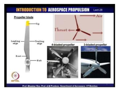
For example, propellers create thrust essentially by harnessing the air, which is available in the atmosphere. So, propeller works in the open atmosphere unlike an engine, which works inside an enclosed atmosphere, in an enclosed chamber of an engine. Whereas, the propeller is out in the open, it is working medium is the atmospheric air, the open air.
