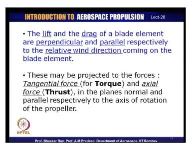
We are using airfoil sections for creation of the propeller blades. Airfoils fundamentally create lift and drag; they are fundamentally shaped to create lift and drag. Lift is the positive component, which we want; drag is the penalty you pay in the process of creation of lift.
