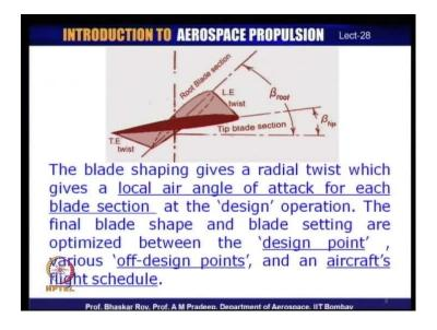
Let us see how airfoils actually are stacked in a blade. Typically when a blade is operational, the lift creation depends on the way the flow is locally incident on the airfoil. It depends on the airfoil characteristic, which is often decided by the local angle of attack.
