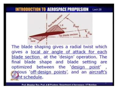
The rotational speed often designated as U, which is equal to omega r - of each blade element, it is different, it varies with r. Omega is fixed from for the entire blade, but the r varies from root to tip, hence that rotational speed would vary from root to tip. As the forward speed is let us say same from root to tip, the pitch setting needs to be varying from the hub to the tip.
