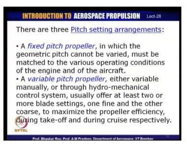
The variable pitch propeller which came a little later actually had the capacity to vary the pitch manually through variable mechanisms, which could be done on ground, during the ground servicing or through some hydro mechanical control system. This could be done
