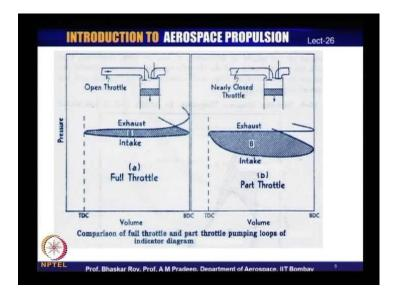
Now, as it is, as we have seen in the earlier diagram, the part throttle condition, the actual operational power available is actually on the lower side. Then, if the power lost in the process of intake exhaust is of much higher order, this could happen due to the fact that the opening of the intake valve could be earlier or closing of the exhaust valve could be earlier.
