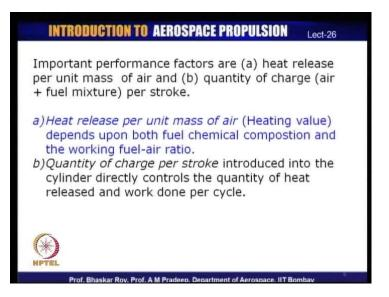
The important performances parameters that we need look into are; the heat release per unit mass of air. This is the quality of the fuel that you are putting into the engine, so the choice of the fuel needs to be taken care of by the heat release capacity of this fuel. The other is the quantity of charge, which is a mixture of air and fuel mixed in the carburetor per stroke of the engine.
