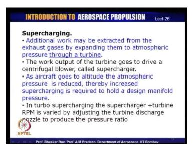
So, the supercharging produces additional work that may be extracted from the exhaust gases by expanding them to the atmosphere through a turbine. So, the question now is how do you run the supercharger, which produces this boosting of intake density and pressure? It is done by a running it with the help of a turbine; the question is how do you run the turbine?
