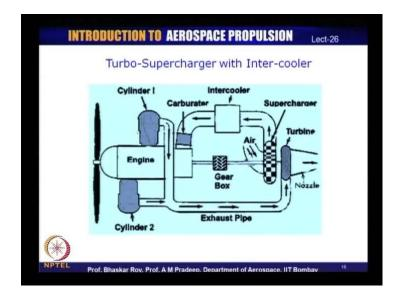
One of the choices that typically an engine designer would have is a turbo supercharger. One of the possibilities is that he can use a turbo supercharger with what is also known as intercooler.
