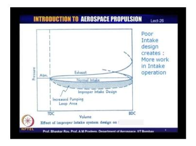
The other issue is the poor intake design. We need to look at the fact that the intake operates ideally at a constant pressure. If the intake operates at a pressure much lower than what it is scheduled to, we get inlet intake loop that is now much bigger than what it should have been ideally. This intake loop now takes away work from the main engine in the process of pumping as it shown here, this extra intake pumping work now, is not available as an engine output.
