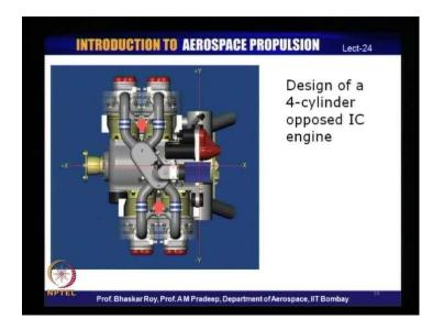
This is a design of a four cylinder opposed IC engine, which shows the internal parts of the four cylinder IC engine. It powers one single crank shaft and powers propeller, so this shows all the details of cut out of typical four cylinder opposed IC engine.
