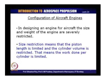
Now, this means that you would require a piston, which is of larger size or longer in length to obtain higher efficiency. Now, this a bit of a problem that in an aircraft, if you are looking at anything that has to go on a flying aircraft, the size and weight are restrained, they are premium. Because, anything that you carry in an aircraft would have to be compensated for, by creating more thrust.
