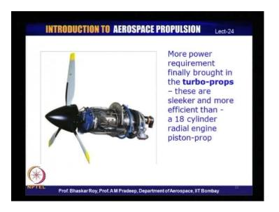
Once the amount of engine power required goes up, we have seen that you could have 6 cylinders, you could have 8 cylinders, you could have 10 cylinders, you could have 9 cylinders and you have 9 in to 2, so18 cylinders. So, there are engines - piston-prop engines, where up to 18 cylinders have been put together to power an aircraft.
