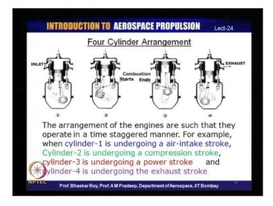
Now, let us look at an arrangement of cylinders, let us take say four cylinders - the kind of thermodynamic arrangement that we have. We have four stroke engines, so let us say that we have four cylinders, let us look at the four strokes that it has to undergo.
