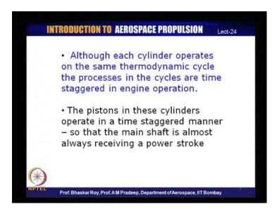
As we have seen, in the earlier one, each of these pistons actually operates under a particular thermodynamic cycle. Thermodynamic cycle is the basis on which each of these pistons is actually working.
