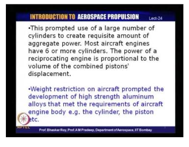
Now, as a result of the fact, to make an aircraft fly, you need certain aggregate amount of power. To use this aggregate amount of power, you need to then put together a number of cylinders, so that the aggregate amount of power is quite sufficient to meet the requirements of aircraft thrust requirement.
