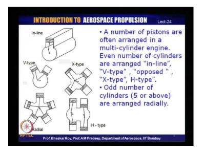
Let us take a quick look again at some of the arrangements that are quite often done in various kinds of aircraft engines, which often tend to be multi cylinder engines. As we seen, the multi cylinder is often arrived at by putting together the total amount of work that is necessary to drive the propeller, which of course creates a thrust that flies the aircraft.
