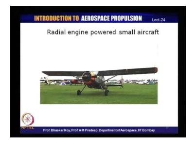
This is the kind of radial engine that often powers a small aircraft. Now, this is the kind of shape that typically a radial engine would have to be housed inside. You would have circular front body of the aircraft within which the radial engine would be housed inside, it would of course drive the propeller.
