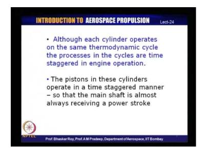
Especially, most of the aircraft do have multi cylinder arrangement, even though each and every of these cylinders is actually operating under same thermodynamic cycle.
