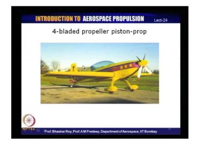
This is a 4-bladed propeller - piston propeller, you can see here that the shape of the aircraft again has dictated the kind of engine it should use. One can make a guess that the engine used here is the opposed type - multi cylinder opposed type, probably 3 in to 3
