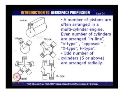
Let us quickly go back to the earlier one. If you can see here, for example, this diagram, the cylinders, as you can see here, are at different positions. These two are more or less at same position; whereas these two are at same position. So, the power stroke of these two are probably time together, whereas the power stroke of these two cylinders are probably time together.
