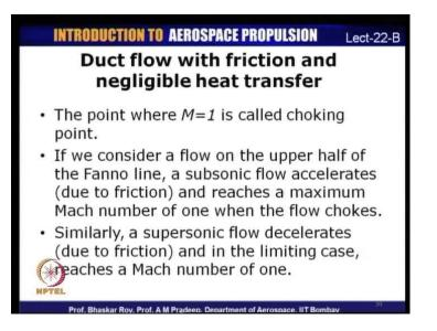
The point where Mach number is 1 is known as choking and so, it is possible that in a subsonic flow, you can accelerate the flow; it basically happens because of friction. In the case of supersonic flow, the flow decelerates and in the limiting case, it reaches a Mach number of 1.
