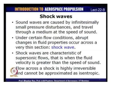
Let us look at what we mean by shock waves. Shock waves are basically certain aspects of a flow in a supersonic flow, where there could be abrupt changes in fluid properties. Now, we have already defined, what is meant by speed of sound. Sound waves are caused by infinitesimally small pressure disturbances and they travel through a medium at the speed of sound.
