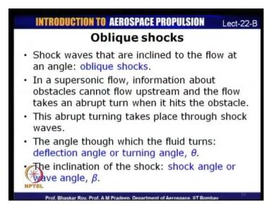
Shock waves that are inclined to the flow at an angle are basically known as oblique shocks. Why do we have an oblique shock in the first place? We have already seen why normal shocks occur; the same reason applies for an oblique shock as well and in a supersonic flow, the presence of obstacles cannot be felt by the flow which is upstream.
