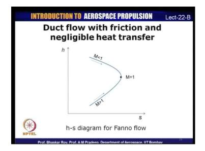
On a h-s diagram, we can represent a Fanno line similar to that of a Rayleigh line. That is, in a supersonic flow because of friction, entropy is increasing. There is no heat transfer and due to friction, the Mach number increases and in the limiting case, it reaches Mach number equal to 1.
