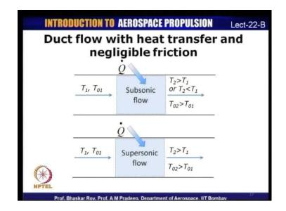
What happens in a Rayleigh line process is that if the Mach number is subsonic and if it is subsonic flow then for a given or predefined temperature upstream, downstream stagnation temperature increases because you are adding heat. So, stagnation temperature has to increase, static temperature may increase or decrease, depending upon where you are on the Rayleigh line; this is on a subsonic flow.
