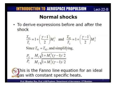
If you have to derive expressions before and after the shock wave, the flow is isentropic before the shock wave and so, we have T 01 by T 1 is equal to 1 plus gamma minus 1 by 2, M 1 squared, where M 1 is the upstream Mach number, T 01 is stagnation temperature upstream and T 1 is static temperature upstream.
