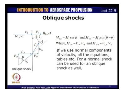
The same set of vectors or the same diagram, if it is tilted and made normal. In the previous case, the oblique shock was inclined at a certain angle, now if we tilt it and make this normal what we get is the following.
