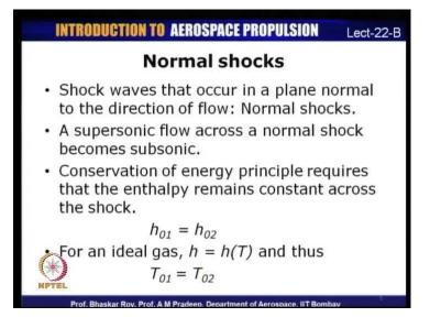
So, downstream of the normal shock, the flow becomes subsonic. Let us look at what are the features of a normal shock wave. Shock waves that occur in a plane which is normal to the direction of the flow are called normal shocks.
