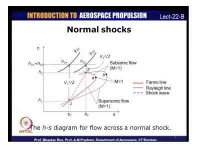
Let me illustrate that through an h-s diagram. On this h-s diagram, you can see that I have plotted the Fanno line equation as well as the Rayleigh line equation. The Fanno line equation is shown by the red line and the Rayleigh line equation is shown by the blue line.
