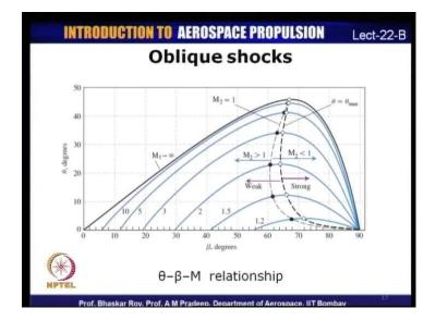
If we do that, we have a chart or a graph or a plot for theta, beta, M, where we have the deflection angle theta on the y axis, the shock angle beta on the x axis and Mach numbers - different contours of the constant Mach numbers.
