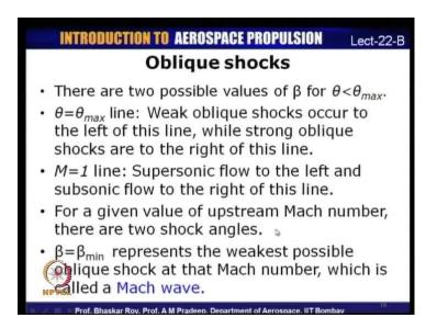
For different values of Mach number, what we can understand from this chart of theta, beta, M is that there are basically two possible values of beta, for any value of theta which is less than theta max. So, if we look at the theta is equal to theta max line, these are lines on the left of which we have weak oblique shocks and on the right of this line, we have strong oblique shocks.
