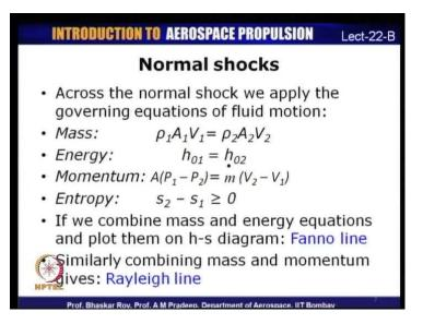
Basically, what we will try to do is to apply the governing equations of fluid motion. We have primarily 4, in fact 5, governing equations: equation for mass, energy, momentum, entropy and the equation of state. If you take up four of these governing equations, let us look at the mass equation or conservation of mass which states that mass flow rate before the shock and after the shock should be the same.
