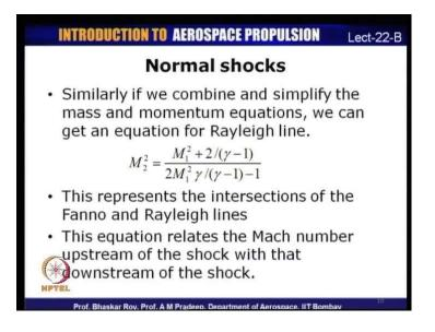
Similarly, we can combine and simplify the mass and momentum equations and what we get is an equation for Rayleigh line. If we were to combine the mass momentum equations, we basically get the Rayleigh line equation and we correspondingly can relate some of the properties that are upstream and downstream.
