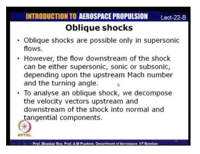
Like we have discussed already for a normal shock, oblique shocks are also possible only in supersonic flows and so, flow downstream of the shock could either be subsonic or it could remain supersonic or it could be sonic and this depends upon the upstream Mach number and the turning angle.
