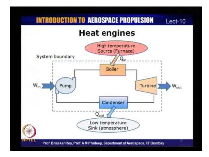
So, heat engine can be actually a multi component cycle. Now, I am explaining the same example here in the case of I mentioned about the steam turbine unit, which is illustrated here. So, what you see, what you saw here denoted by heat engine is shown in the form of is basically the system boundary here as indicated. It could consist of let us say in this example we have four components. There is a turbine; there is a condenser, a pump and a boiler.
