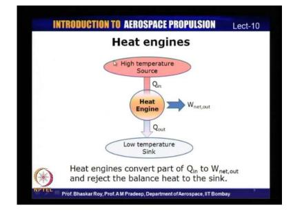
So, what is shown here is a schematic of a heat engine. So, heat engine is something which operates between a high temperature source which is a thermal energy reservoir, and it, the other end of the heat engine is a low temperature sink which is yet another thermal energy reservoir which is a sink.
