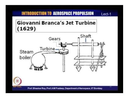
The problem of course was not just making an aircraft, powering the aircraft. To power an aircraft, it is necessary to have engines. When we talk about propulsive devices, we are talking about a devices have an embedded engine inside it. Now, this engine works often on the principle of thermodynamics as we have seen, but the mechanical sciences that do come in the process of propulsive devices involve a number of elements.
